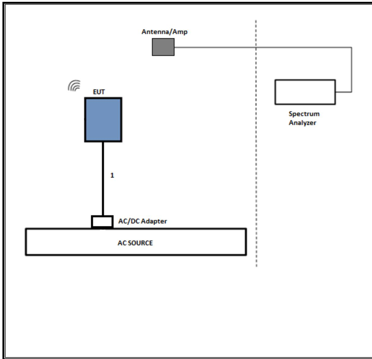
**SETUP DIAGRAM FOR LINE CONDUCTED TESTS**
