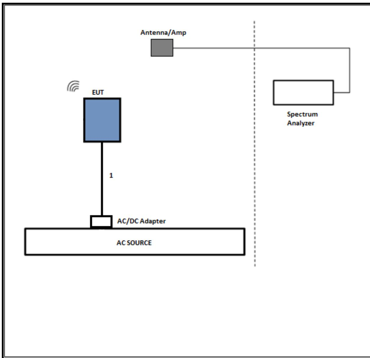
**SETUP DIAGRAM FOR LINE CONDUCTED TESTS**
