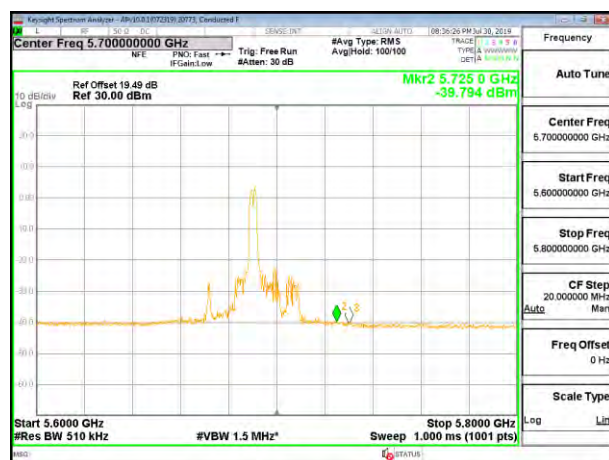
CHANNEL 138 PSD ANTENNA 5
