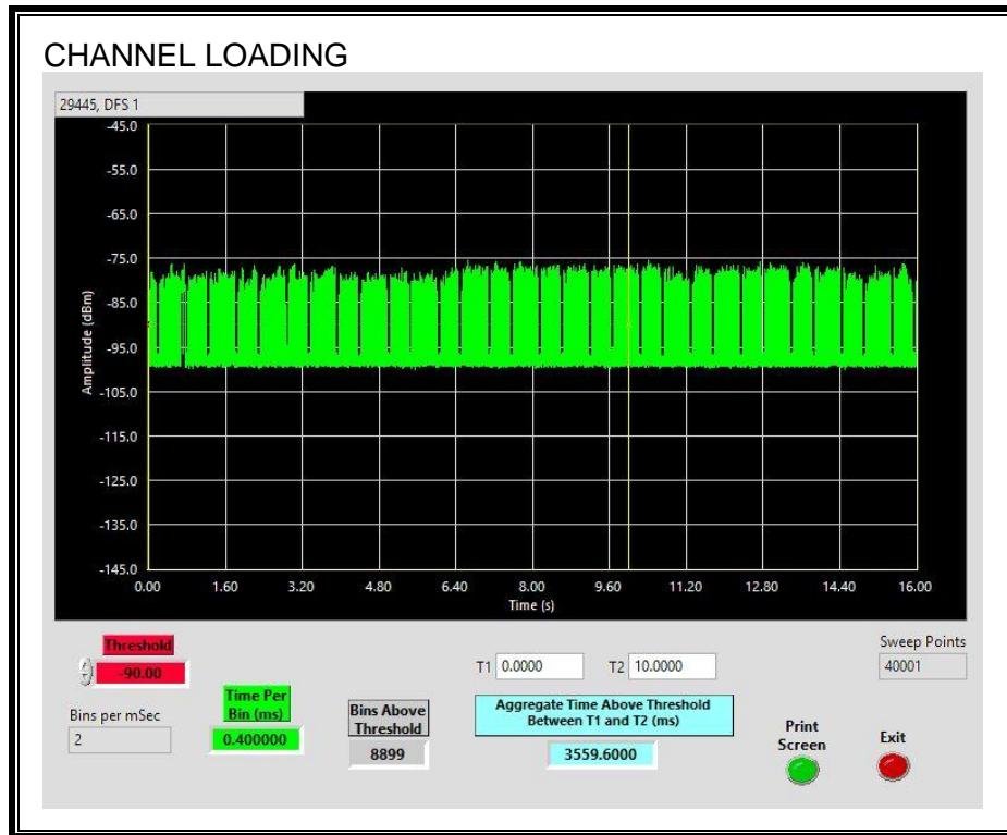
The level of traffic loading on the channel by the EUT is 35.59%
