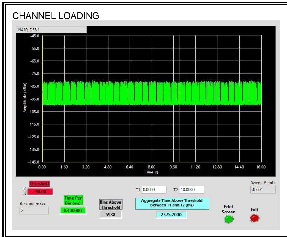
The level of traffic loading on the channel by the EUT is 23.75%
