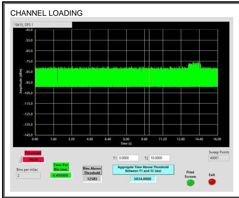
The level of traffic loading on the channel by the EUT is 50.34%
