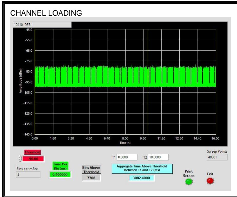
The level of traffic loading on the channel by the EUT is 30.82%
