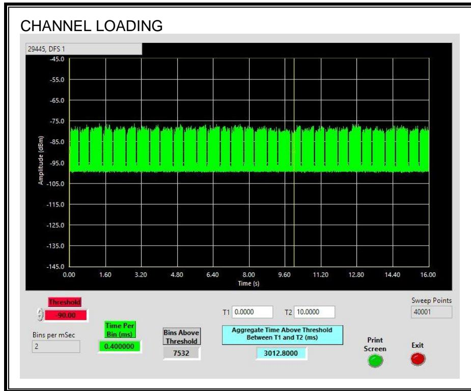
The level of traffic loading on the channel by the EUT is 30.12%
