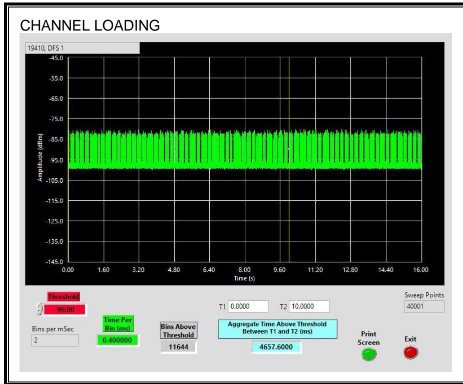
The level of traffic loading on the channel by the EUT is 46.57%
