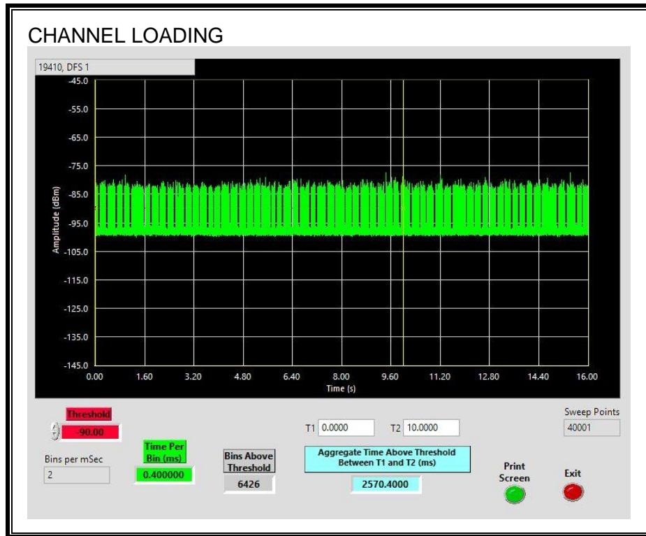
The level of traffic loading on the channel by the EUT is 25.70%
