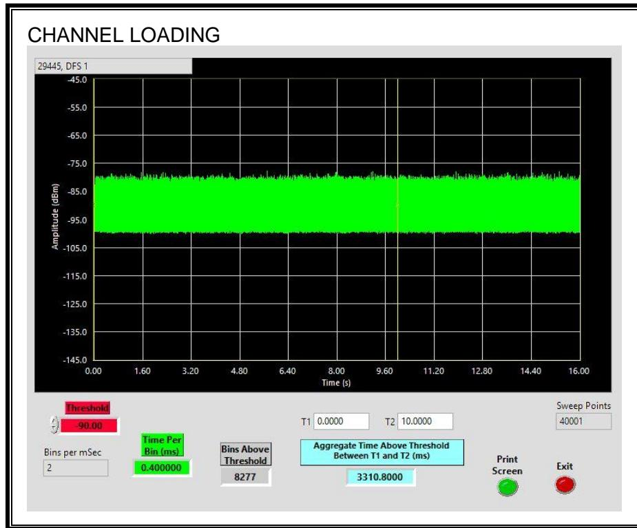
The level of traffic loading on the channel by the EUT is 33.10%
