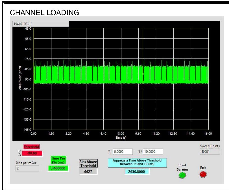
The level of traffic loading on the channel by the Peer Slave is 26.50%
