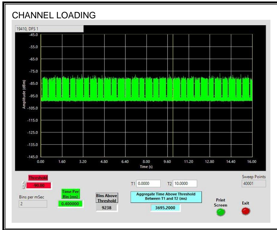
The level of traffic loading on the channel by the EUT is 36.95%
