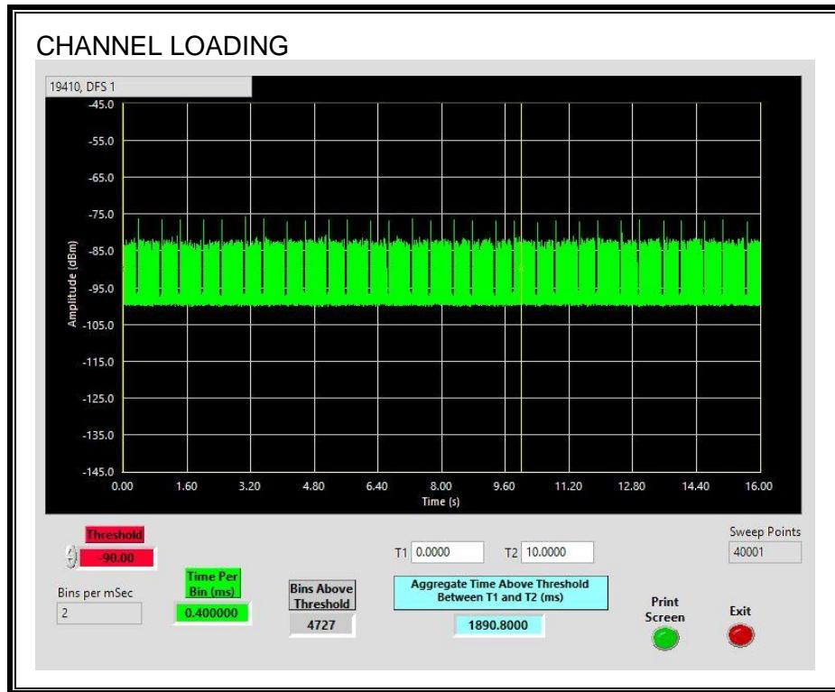
The level of traffic loading on the channel by the Peer Slave is 18.90%
