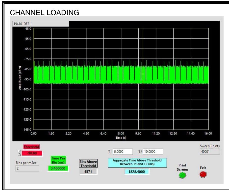
The level of traffic loading on the channel by the Peer Slave is 18.28%
