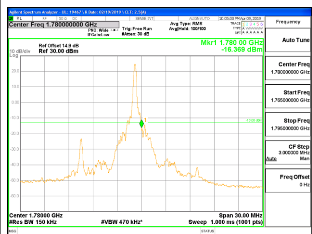
LTE B66 15MHz QPSK High Channel RB1-74
