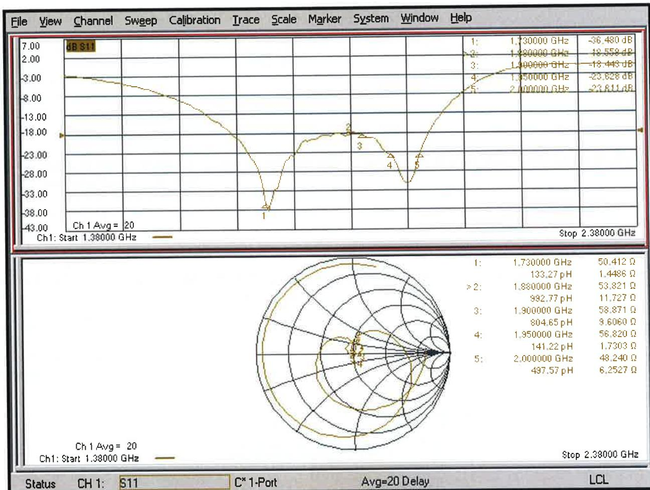
**Dipole E-Field measurement @ 1880MHz/E-Scan - 1730MHz d=15mm/Hearing Aid Compatibility Test (41x181x1):**
