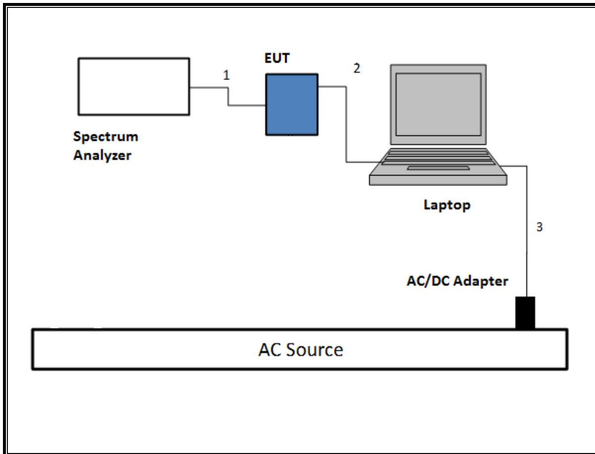
**SETUP DIAGRAM FOR RADIATED TESTS Above 1 GHz**
