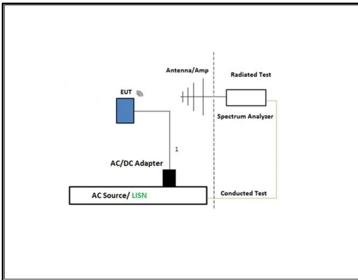
**TEST SETUP- AC LINE CONDUCTED: LAPTOP CONFIGURATION**
