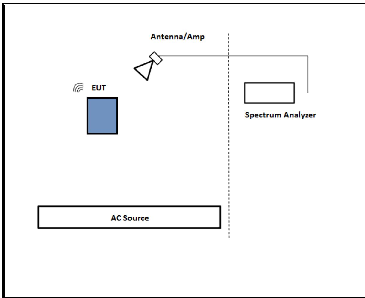
**SETUP DIAGRAM FOR Below 1GHz and AC LINE CONDUCTED TEST**
