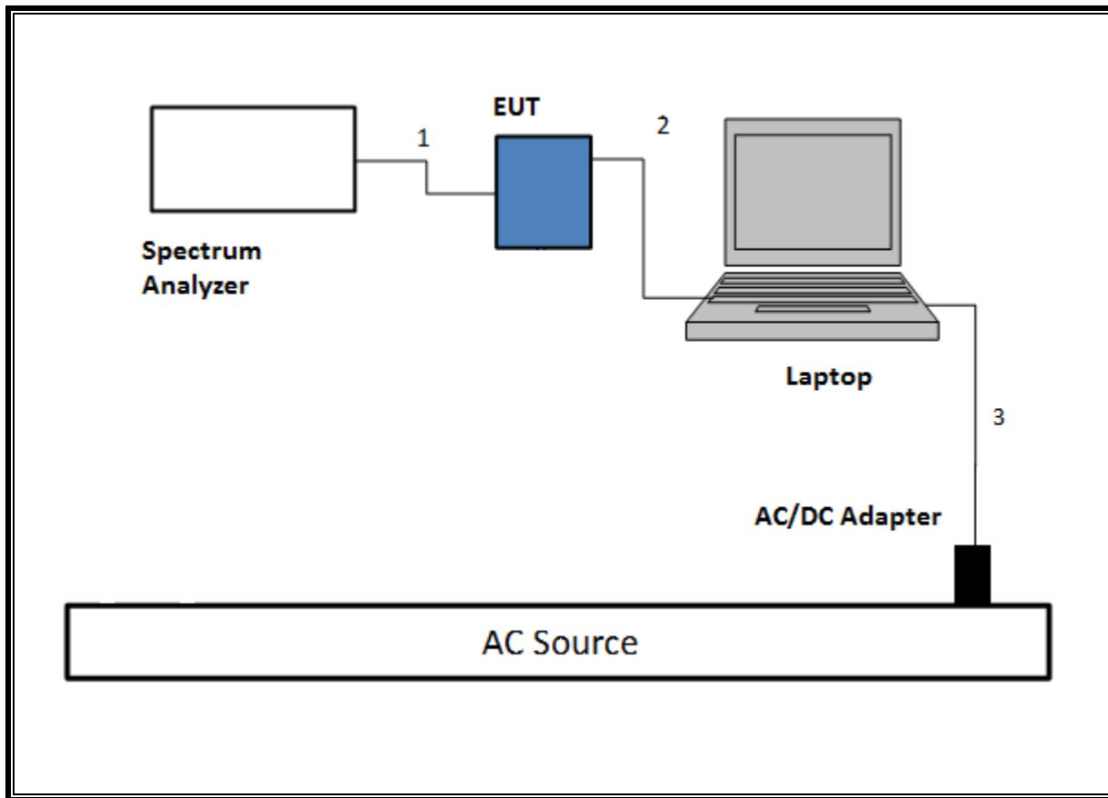
**SETUP DIAGRAM FOR RADIATED TESTS Above 1 GHz**
