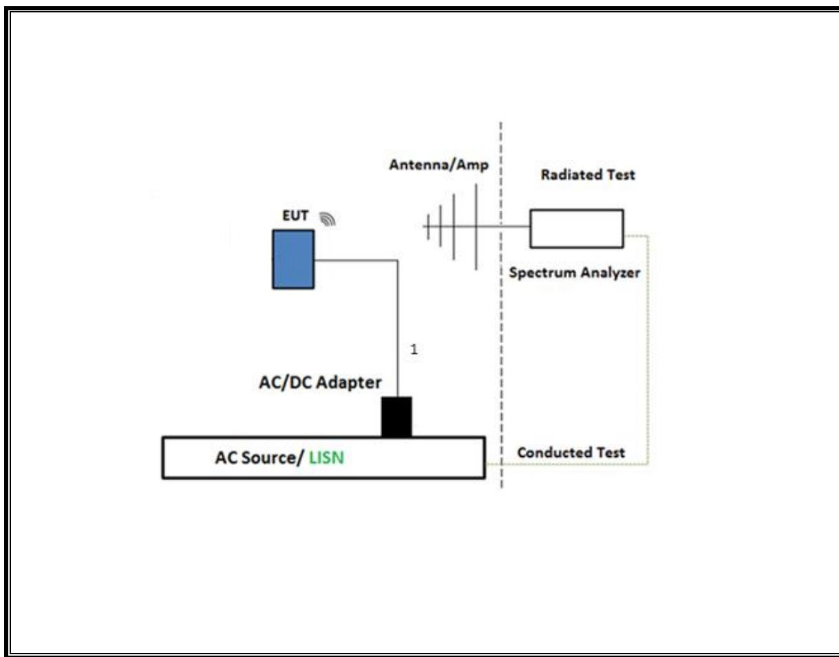
**TEST SETUP- AC LINE CONDUCTED: LAPTOP CONFIGURATION**
