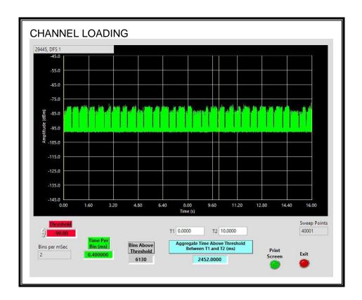
The level of traffic loading on the channel by the EUT is 24.52%
