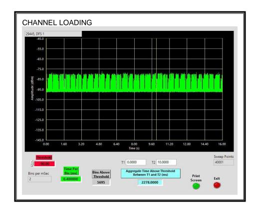
The level of traffic loading on the channel by the EUT is 22.78%
