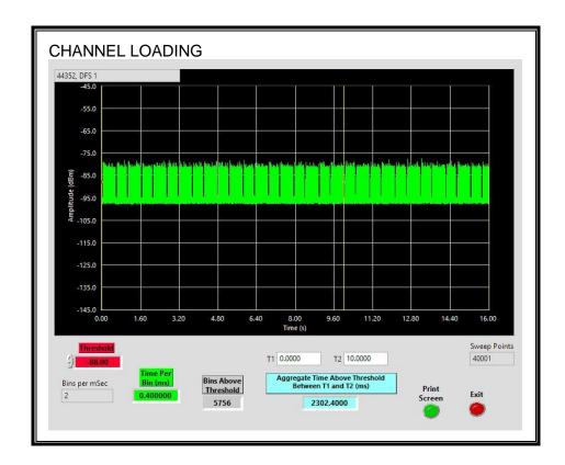
The level of traffic loading on the channel by the Peer Slave is 23.034%.
