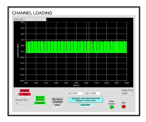
The level of traffic loading on the channel by the Peer Slave is 26.008%.
