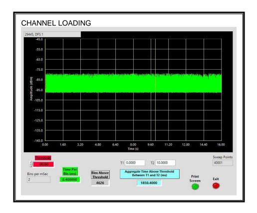
The level of traffic loading on the channel by the EUT is 18.5%
