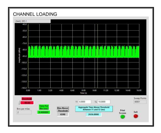
The level of traffic loading on the channel by the EUT is 26.36%
