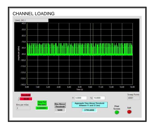
The level of traffic loading on the channel by the EUT is 37.99%
