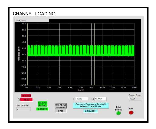
The level of traffic loading on the channel by the EUT is 23.15%
