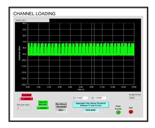
The level of traffic loading on the channel by the EUT is 39.28%
