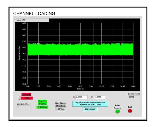
The level of traffic loading on the channel by the EUT is 42.09%
