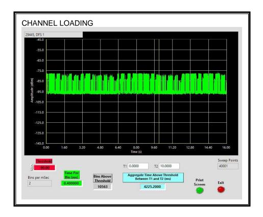
The level of traffic loading on the channel by the EUT is 42.25%
