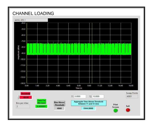
The level of traffic loading on the channel by the Peer Slave is 19.44%.
