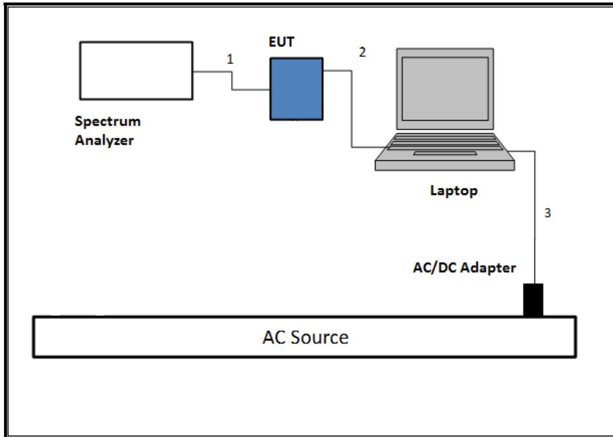
**TEST SETUP- RADIATED-ABOVE 1 GHZ**
