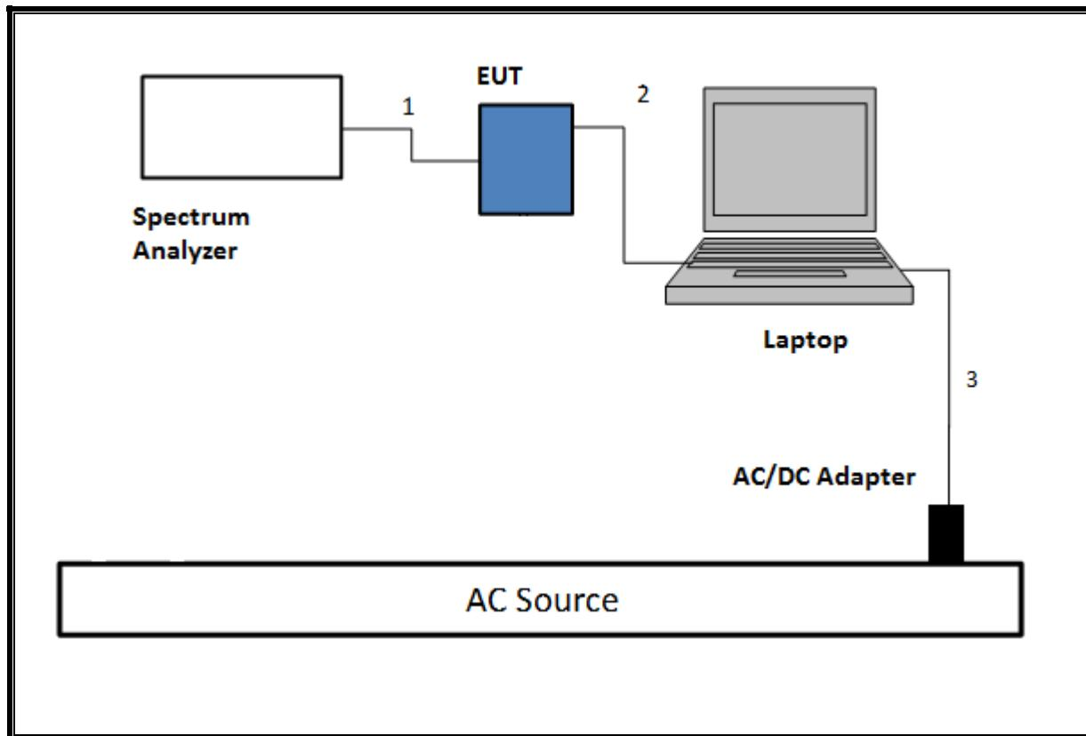
**TEST SETUP- RADIATED-ABOVE 1 GHZ**
