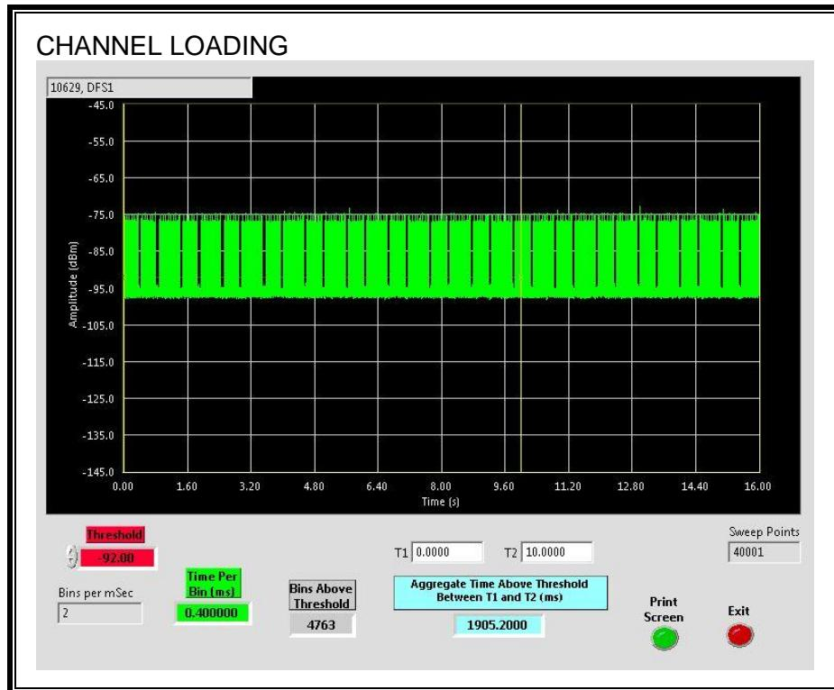
The level of traffic loading on the channel by the EUT is 19.052%
