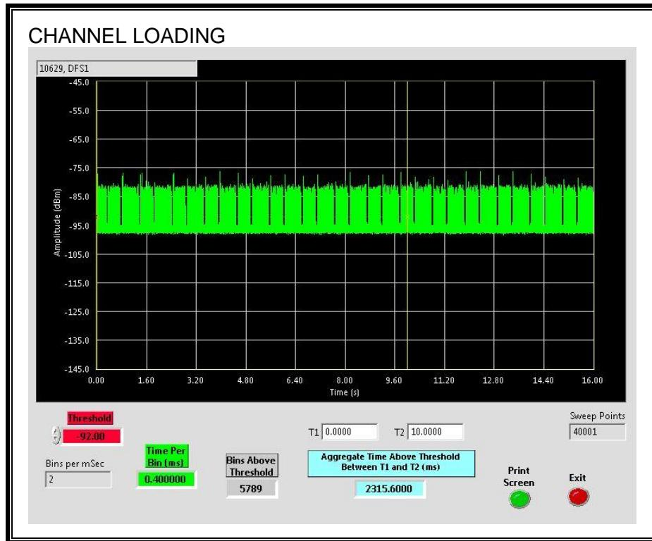
The level of traffic loading on the channel by the EUT is 23.156%
