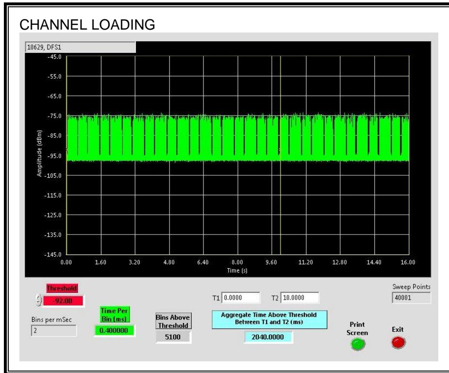
The level of traffic loading on the channel by the EUT is 20.40%
