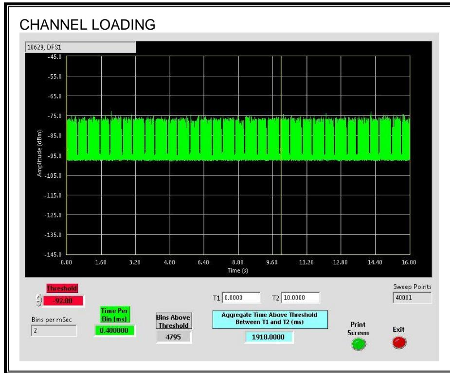
The level of traffic loading on the channel by the EUT is 19.18%
