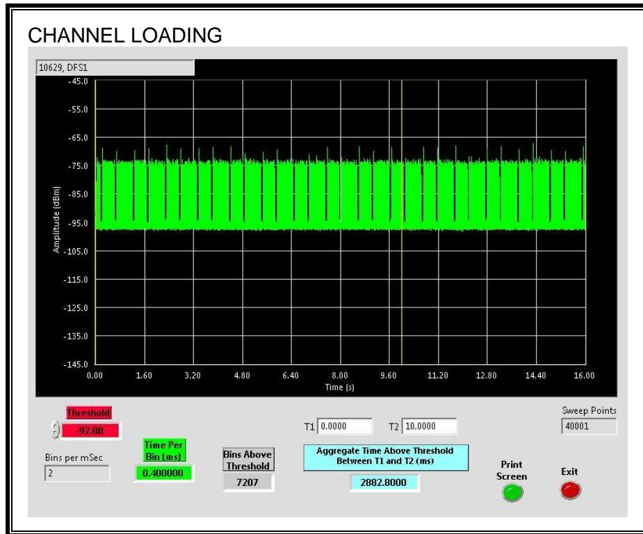
The level of traffic loading on the channel by the EUT is 28.828%
