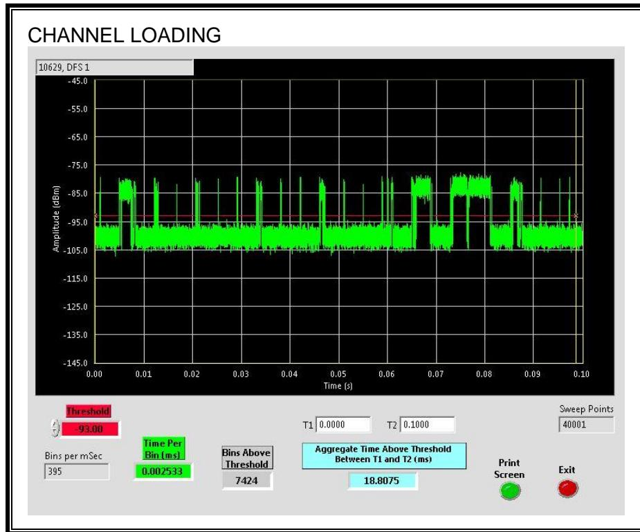
The level of traffic loading on the channel by the EUT is 18.8075%
