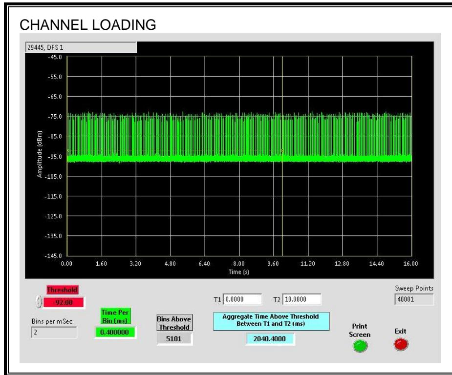
The level of traffic loading on the channel by the EUT is 20.404%
