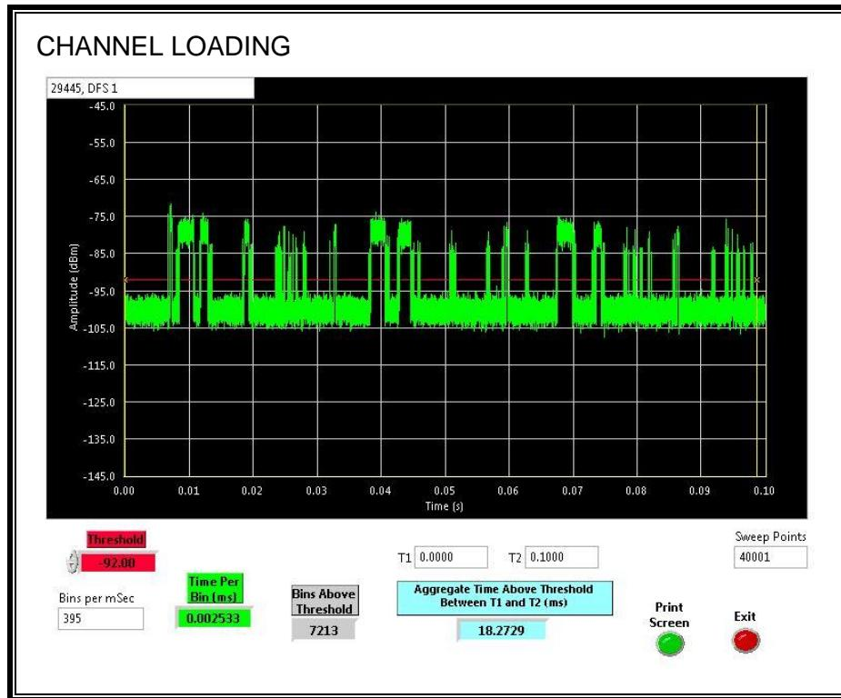
The level of traffic loading on the channel by the EUT is 18.272%
