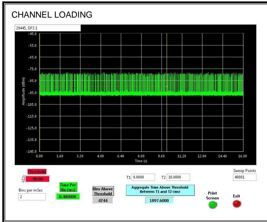
The level of traffic loading on the channel by the EUT is 18.97%
