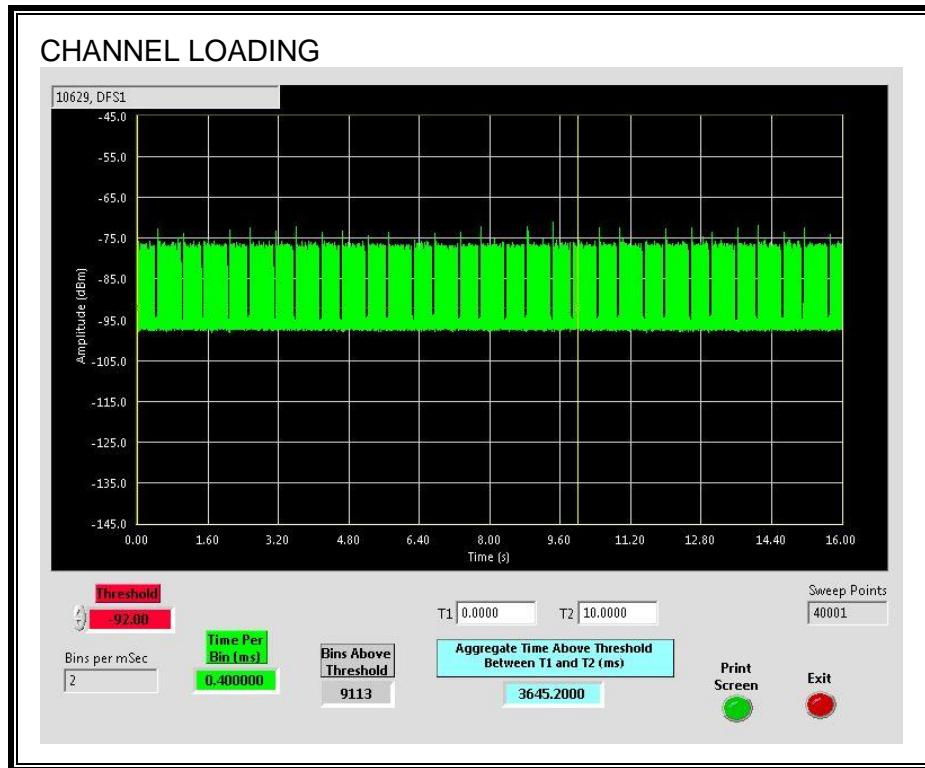
The level of traffic loading on the channel by the EUT is 36.452%
