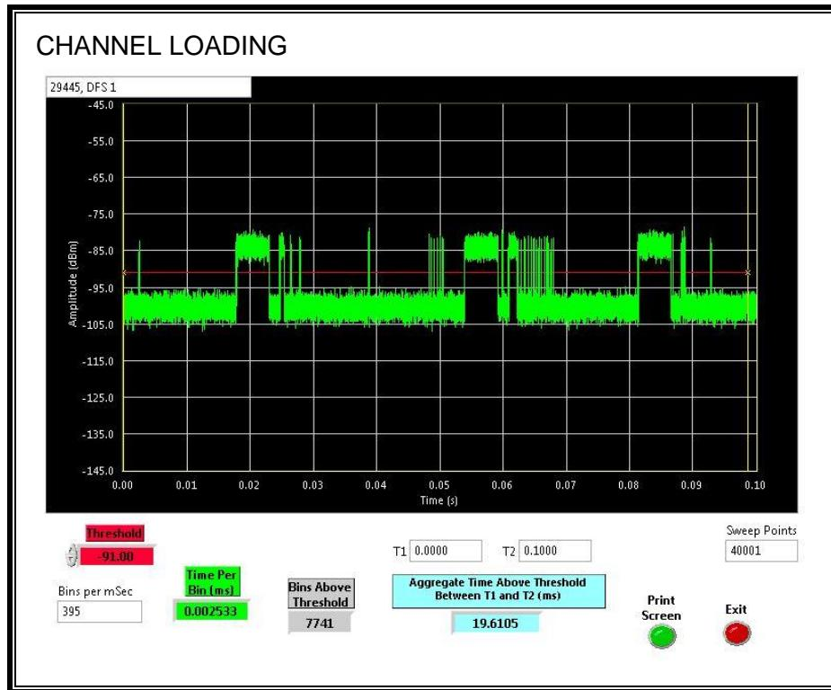
The level of traffic loading on the channel by the EUT is 19.6105%
