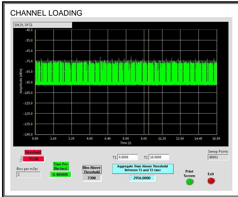
The level of traffic loading on the channel by the EUT is 29.56%.
