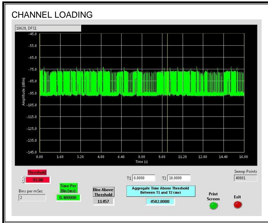
The level of traffic loading on the channel by the EUT is 45.828%
