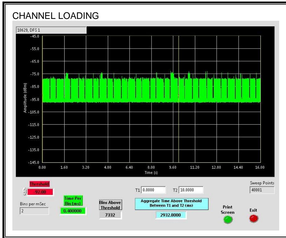
The level of traffic loading on the channel by the EUT is 29.328%
