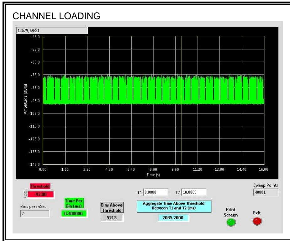
The level of traffic loading on the channel by the EUT is 20.85%
