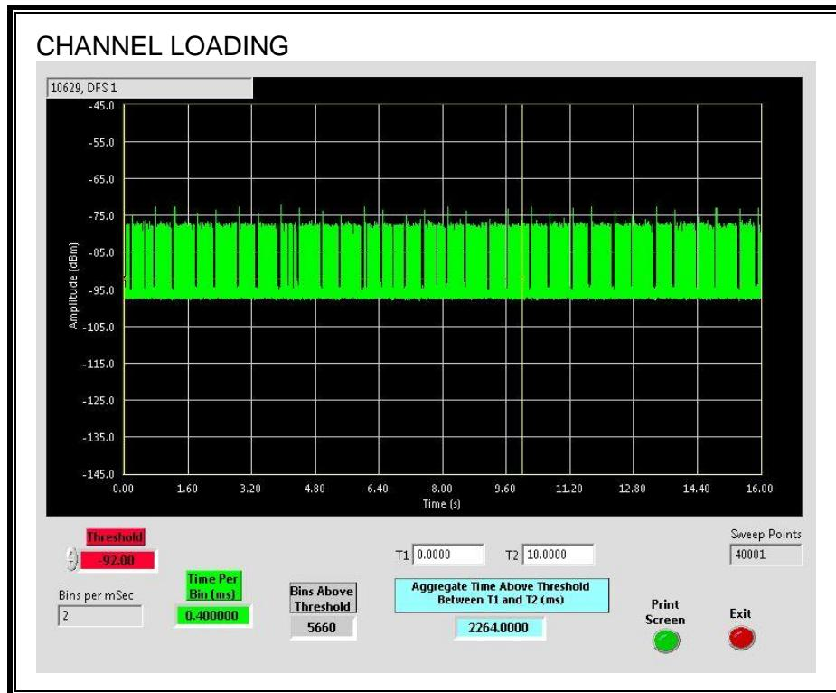
The level of traffic loading on the channel by the EUT is 22.64%
