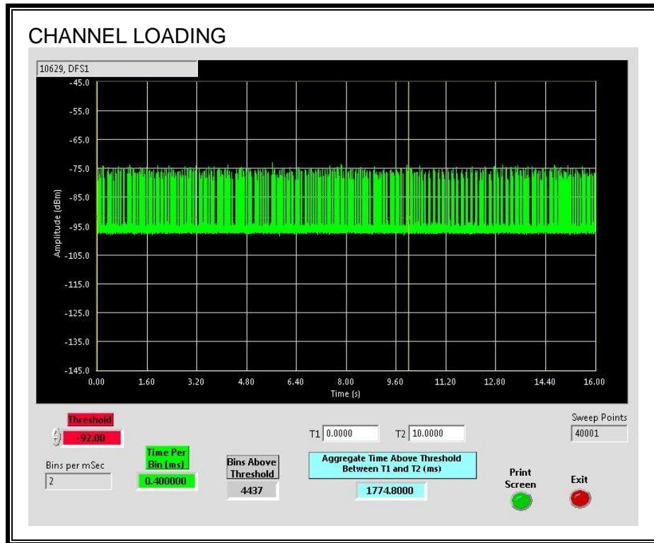
The level of traffic loading on the channel by the EUT is 17.748%
