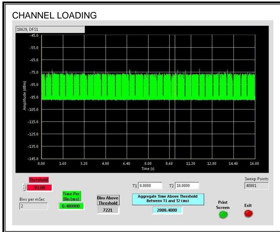
The level of traffic loading on the channel by the EUT is 28.884%.
