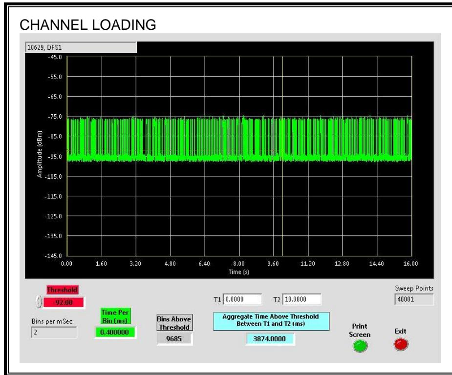
The level of traffic loading on the channel by the EUT is 38.74%
