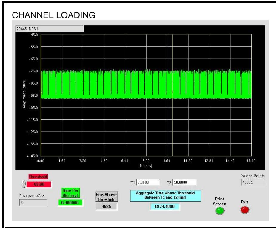
The level of traffic loading on the channel by the EUT is 18.744%
