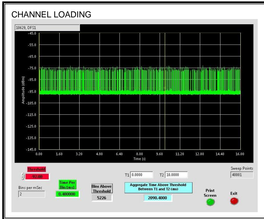
The level of traffic loading on the channel by the EUT is 20.904%
