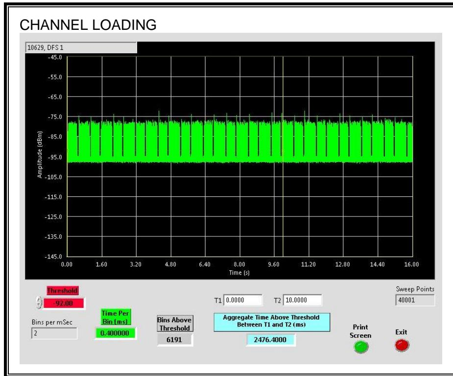
The level of traffic loading on the channel by the EUT is 24.764%
