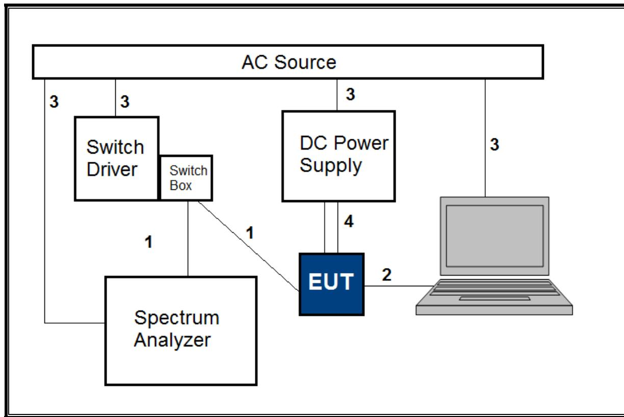
**TEST SETUP- RADIATED-ABOVE 1 GHZ**
