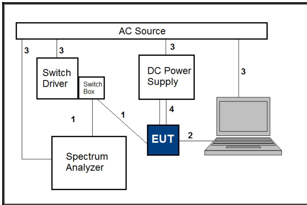
**TEST SETUP- RADIATED-ABOVE 1 GHZ**
