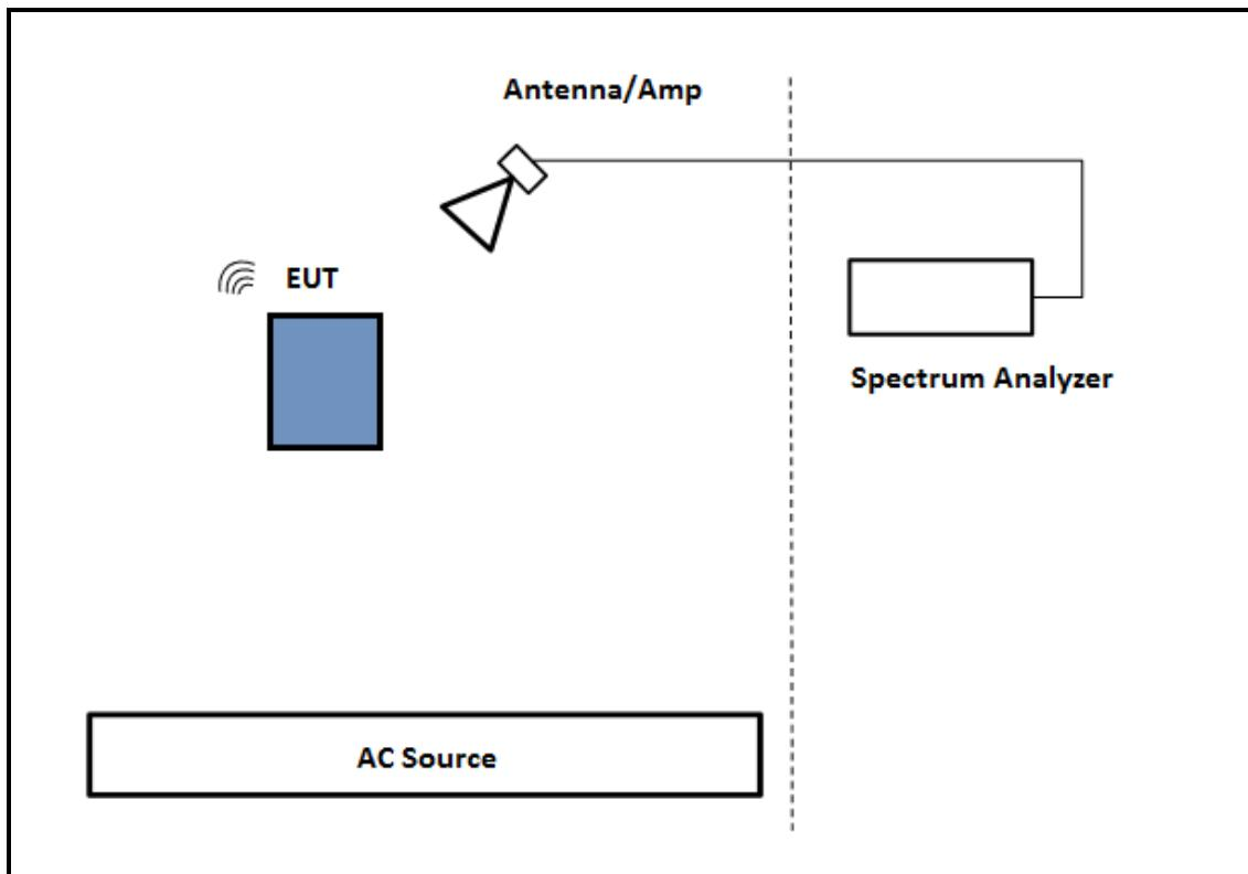
**TEST SETUP- BELOW 1GHZ & AC LINE CONDUCTED TESTS**
