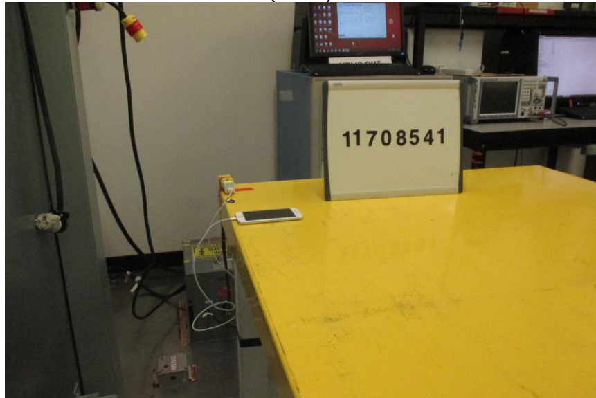
LINE CONDUCTED EMISSION (BACK)
