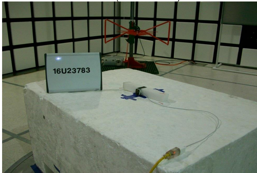
RADIATED FRONT PHOTO (BELOW 1 GHz)
