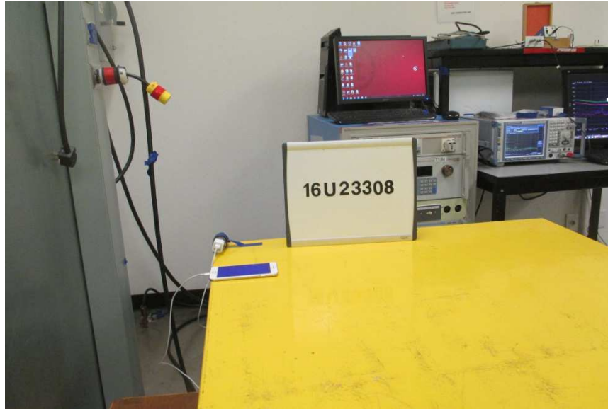
LINE CONDUCTED FRONT PHOTO
