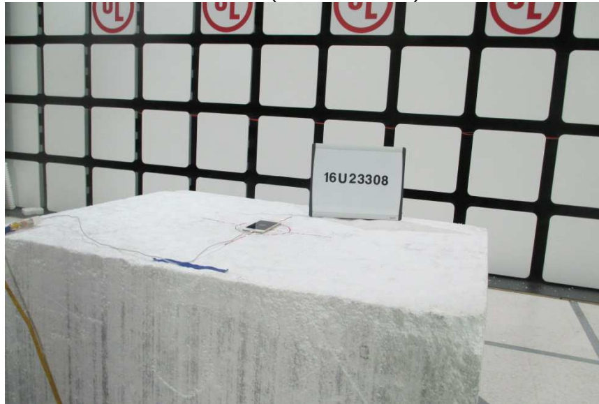
RADIATED FRONT PHOTO (BELOW 1 GHz)
