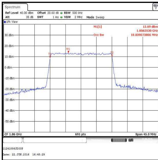
Bottom Channel / 16QAM
