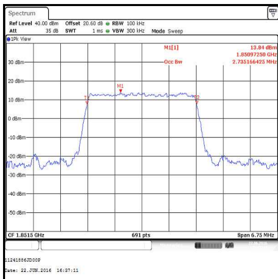
Bottom Channel / 16QAM
