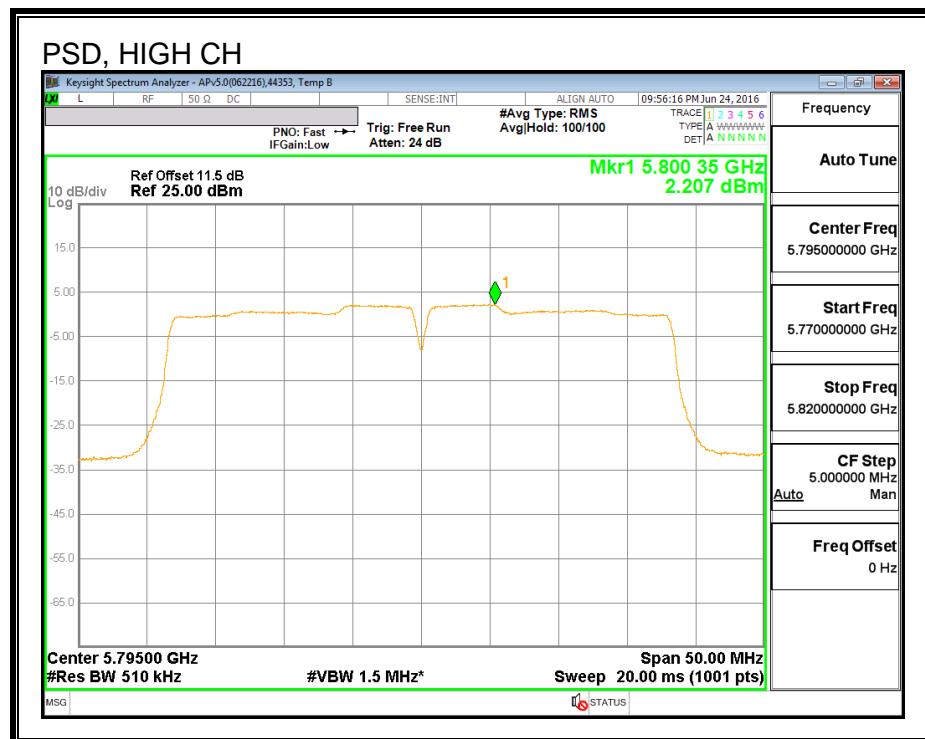
**7.52. 802.11n HT40 CHAIN 1 MODE IN THE 5.8 GHz BAND****7.52.1. 6 dB BANDWIDTH****LIMITS**
