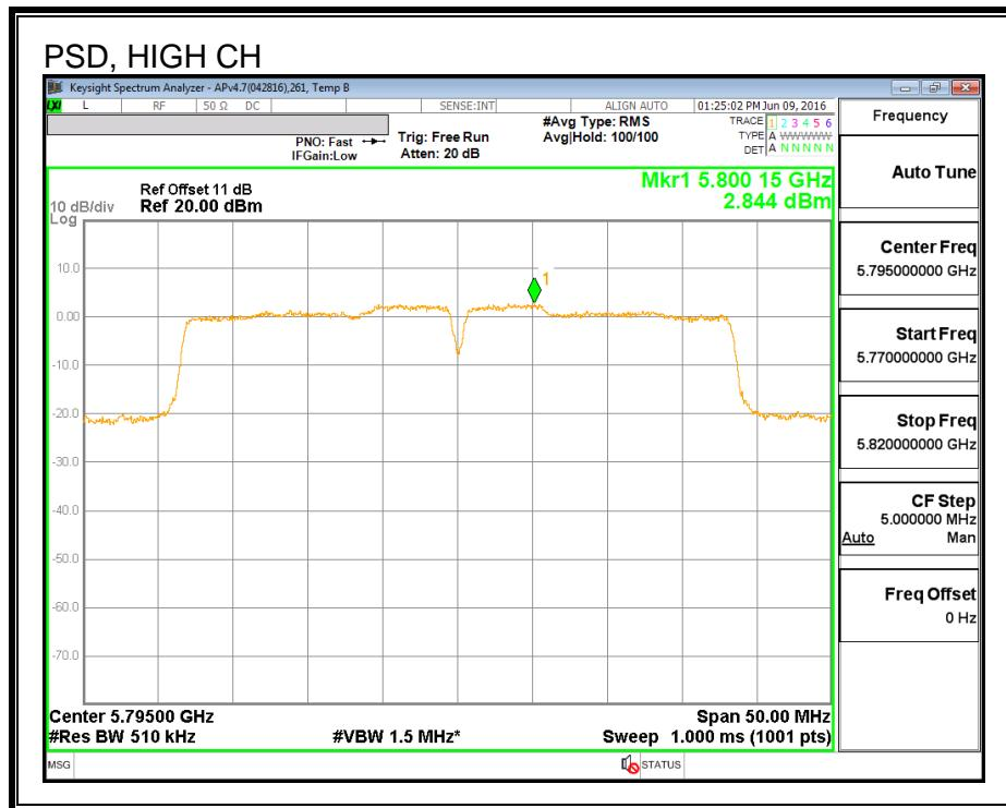
**7.53. 802.11n HT40 2Tx CDD MODE IN THE 5.8 GHz BAND****7.53.1. 6 dB BANDWIDTH****LIMITS**
