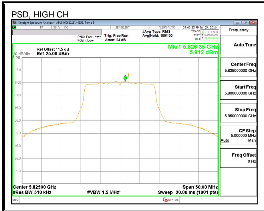
**7.48. 802.11n HT20 CHAIN 1 MODE IN THE 5.8 GHz BAND****7.48.1. 6 dB BANDWIDTH****LIMITS**
