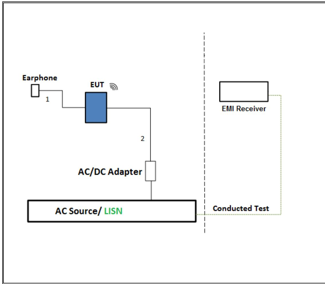
**TEST SETUP- AC LINE CONDUCTED: LAPTOP CONFIGURATION**
