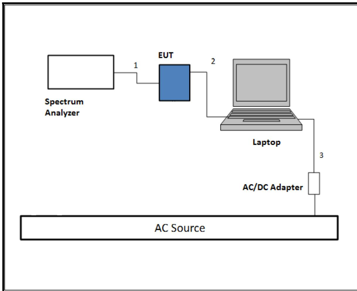
**TEST SETUP- RADIATED-ABOVE 1 GHZ**
