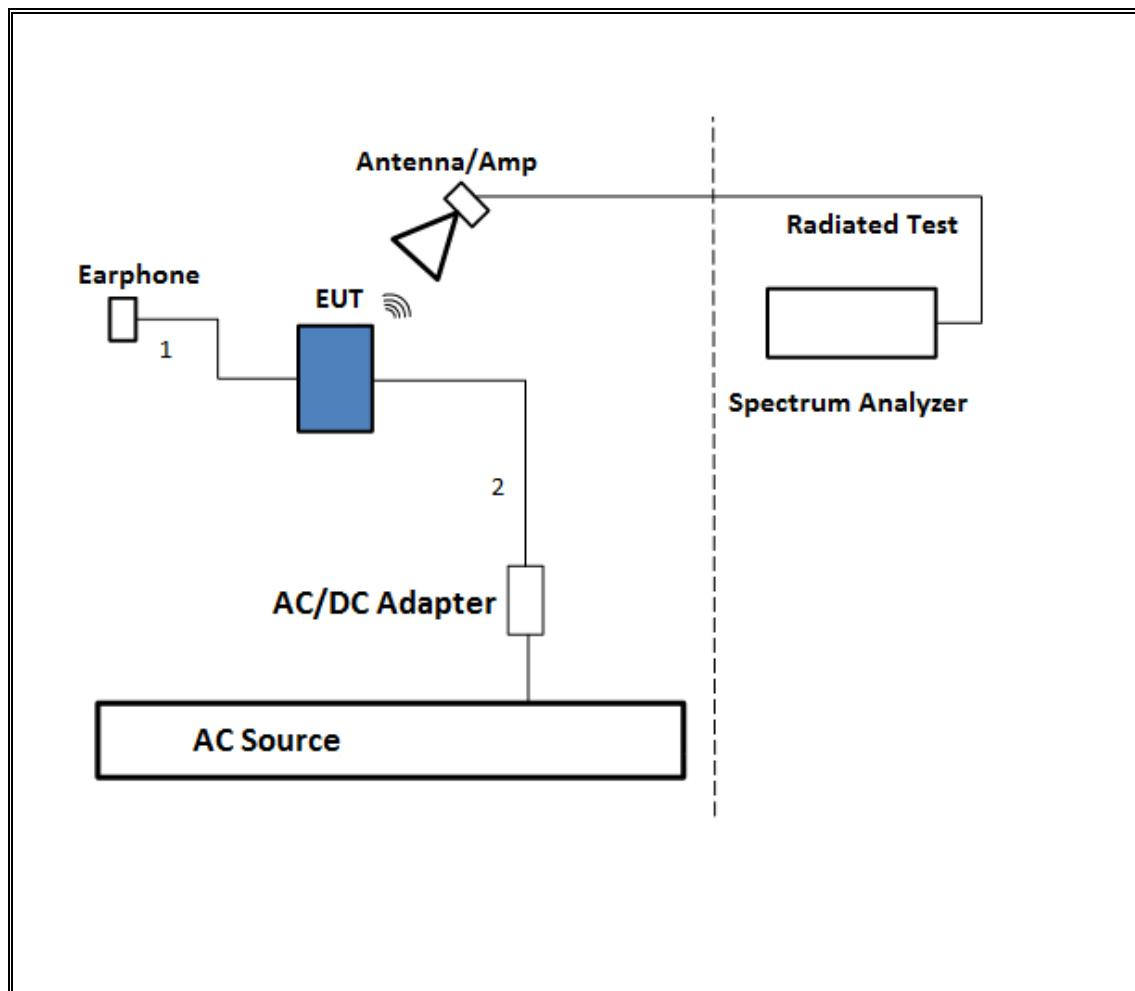
**TEST SETUP- AC LINE CONDUCTED: AC/DC ADAPTER**
