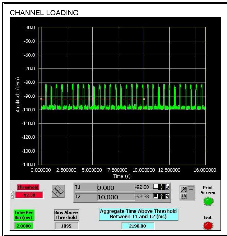
The level of traffic loading on the channel by the EUT is 21.9%
