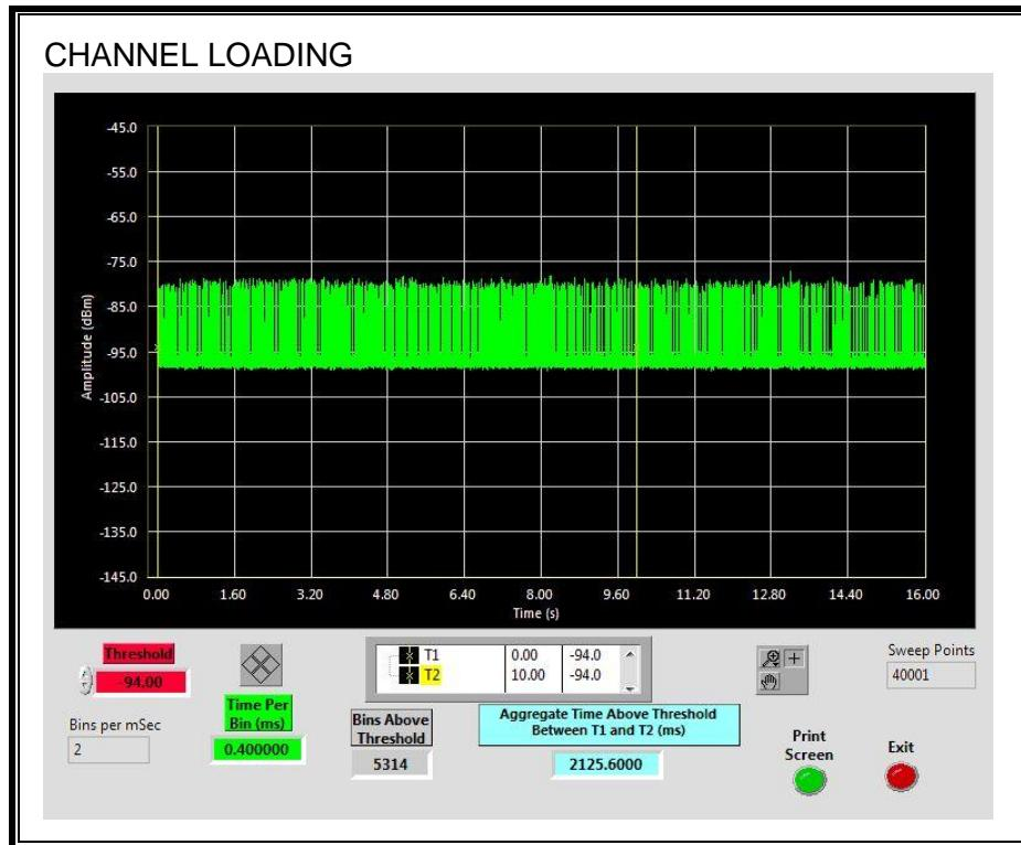
The level of traffic loading on the channel by the EUT is 21.25%
