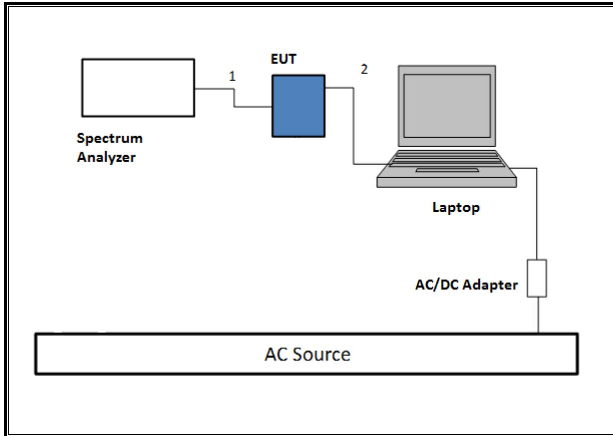
**TEST SETUP- RADIATED-ABOVE 1 GHZ**
