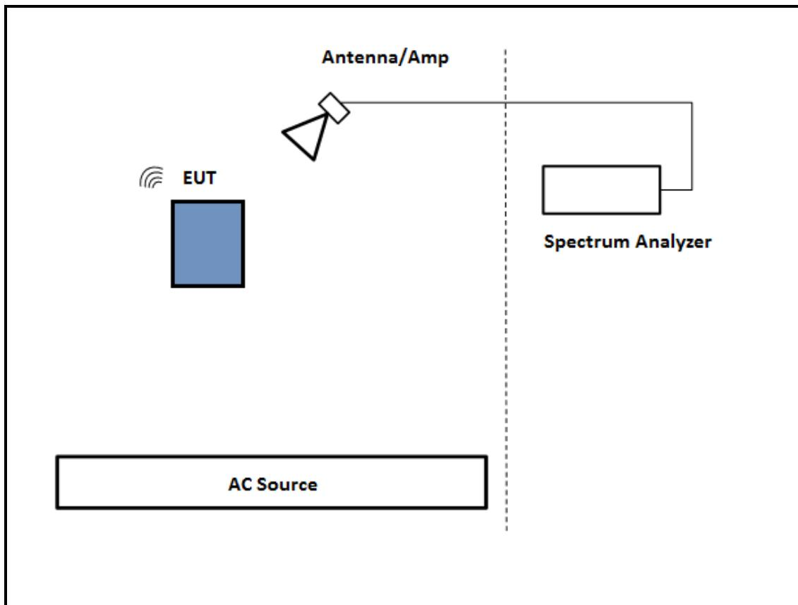
**TEST SETUP- BELOW 1GHZ & AC LINE CONDUCTED TESTS**
