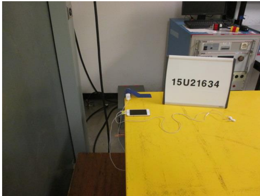
EUT ONLY LINE CONDUCTED BACK PHOTO
