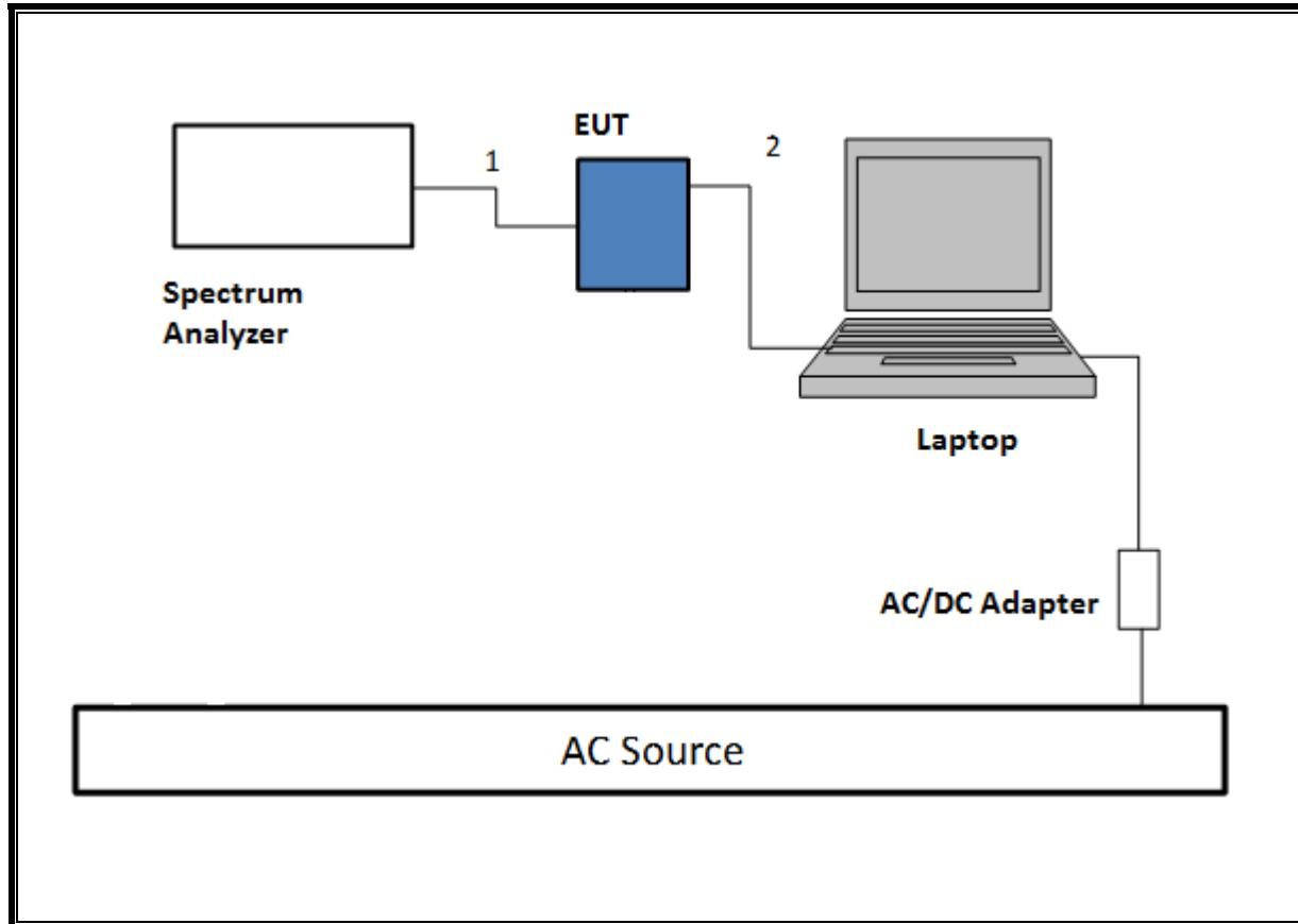
**TEST SETUP- RADIATED-ABOVE 1 GHZ**
