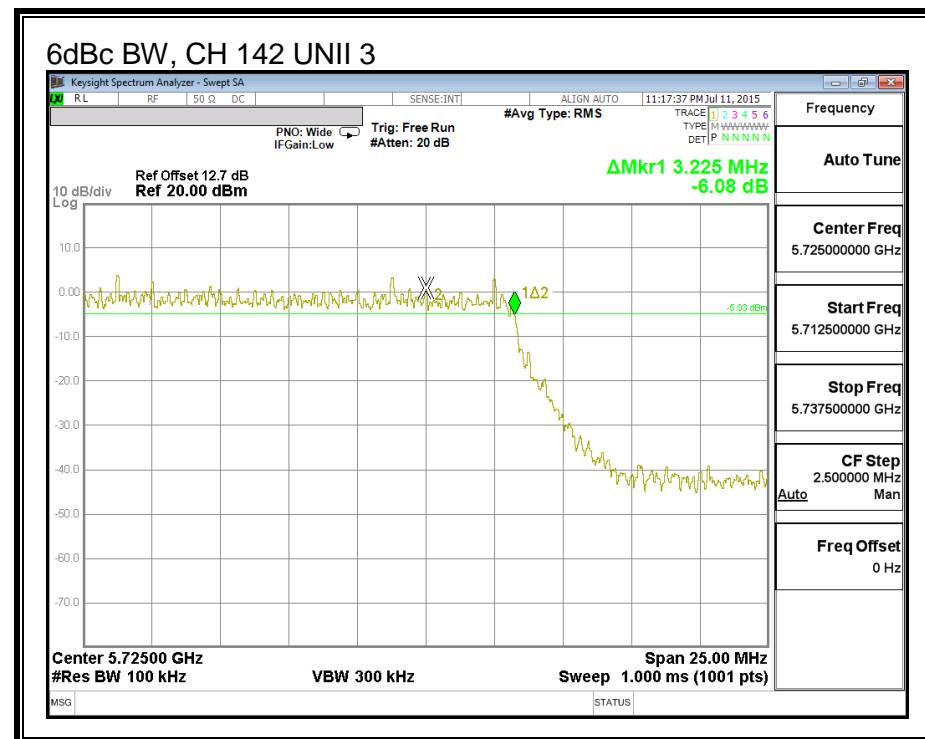
**8.32. 802.11n HT40 2Tx STBC MODE IN THE 5.6 GHz BAND****Note:** Covered by 802.11n HT40 2Tx CDD MODE
