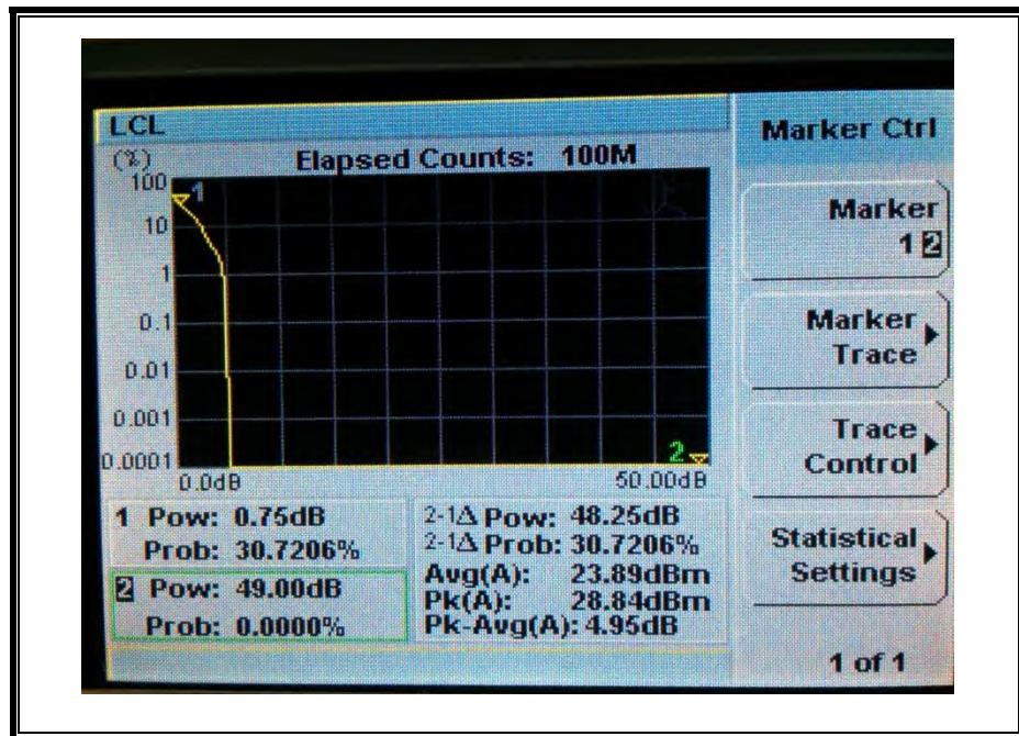
**LTE 16QAM Band 25 (15 MHz BAND WIDTH)**
