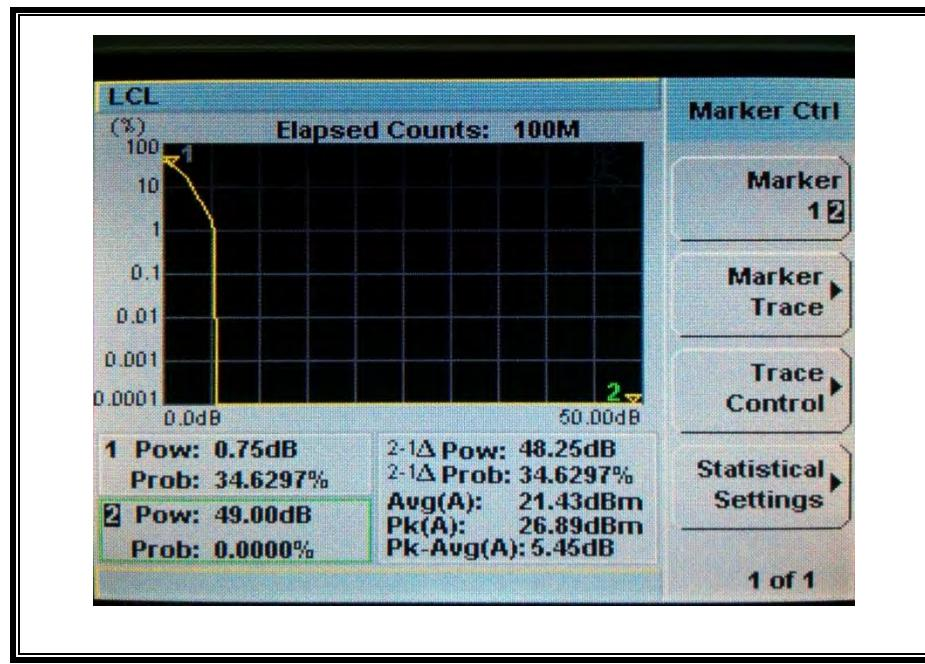
**QPSK Band 26 (5 MHz BAND WIDTH)**
