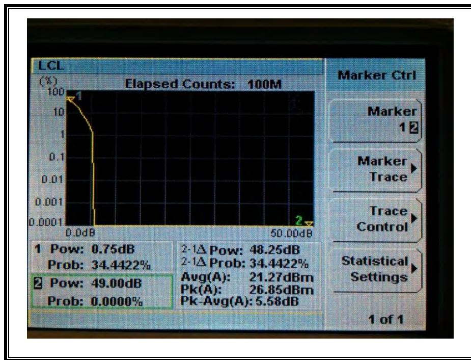
**QPSK Band 26 (10 MHz BAND WIDTH)**
