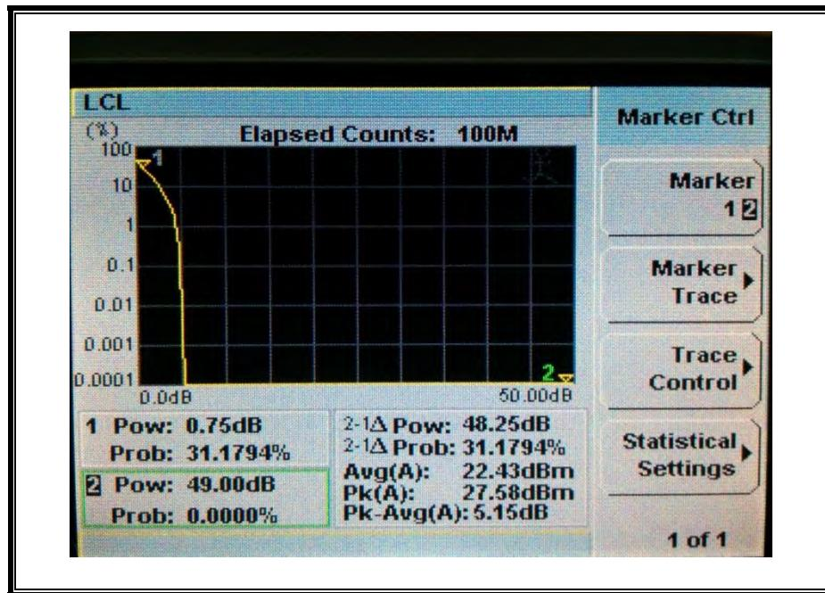
**LTE 16QAM Band 26 (3 MHz BAND WIDTH)**
