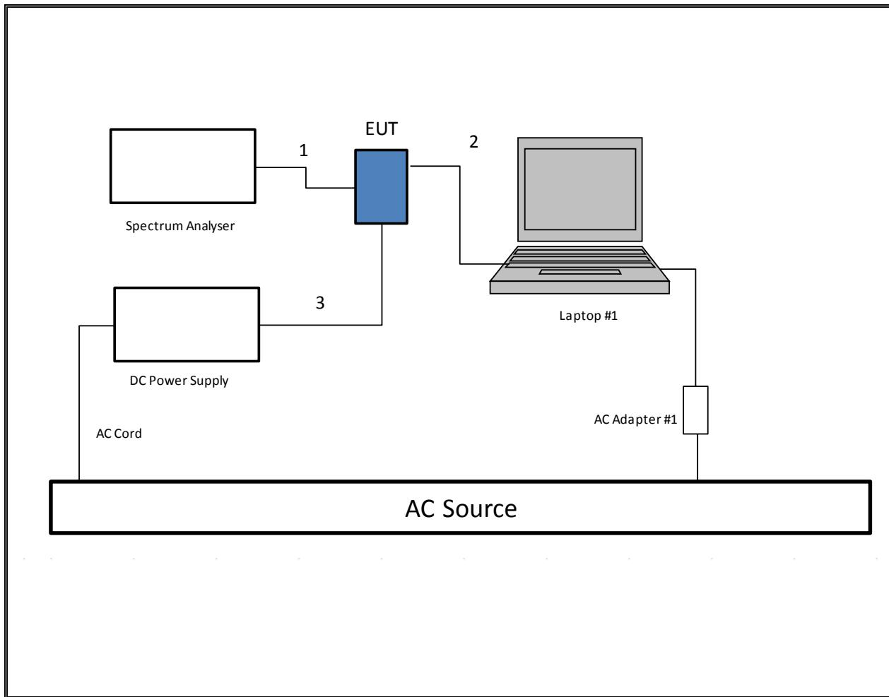
**TEST SETUP- RADIATED-ABOVE 1 GHZ**
