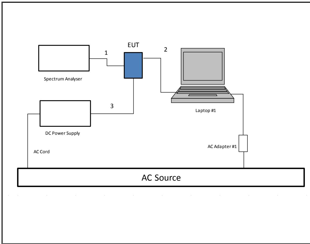
**TEST SETUP- RADIATED-ABOVE 1 GHZ**
