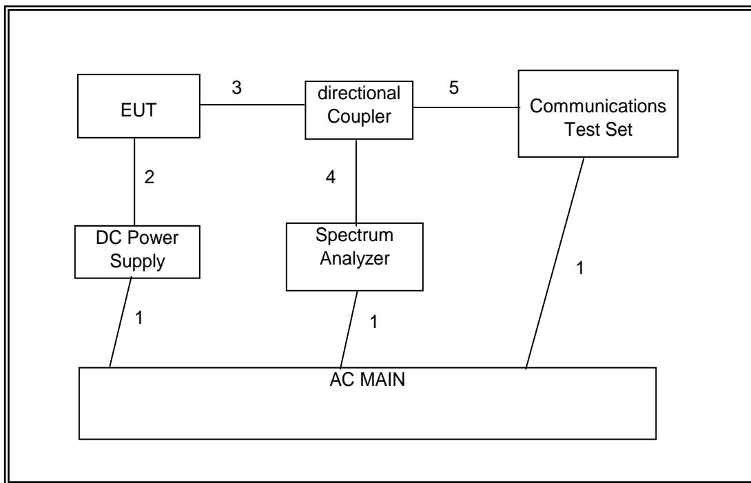
**SETUP DIAGRAM FOR RF RADIATED TESTS**
