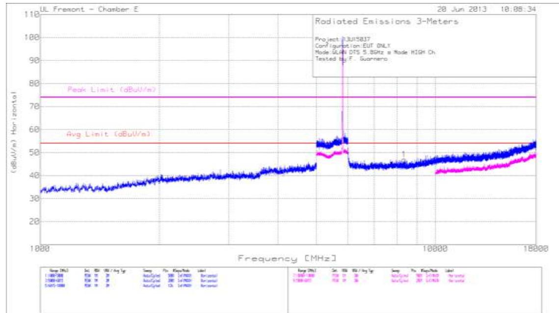
FCC Part15C All 5GHz UNII and DTS Spurious Emissions with Average Scan TSI 38915 19 Jun 2013 Rev. 9.5 13 Jun 2013
