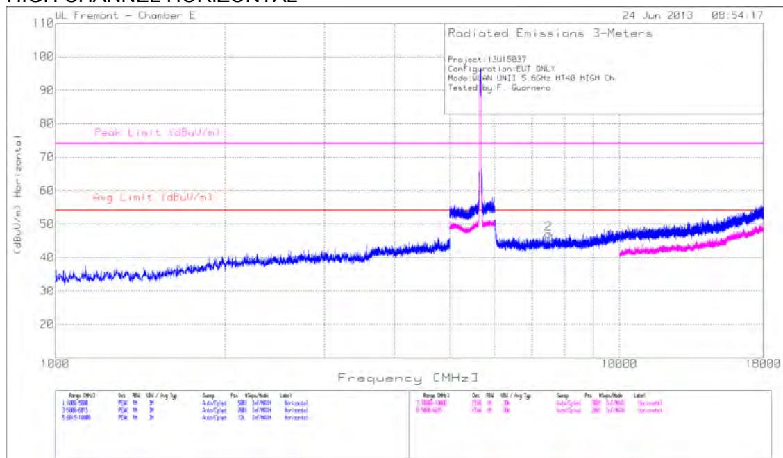
FCC Part15C All 5GHz UNII and DTS Spurious Emissions with Average Scan TST 38915 19 Jun 2013
