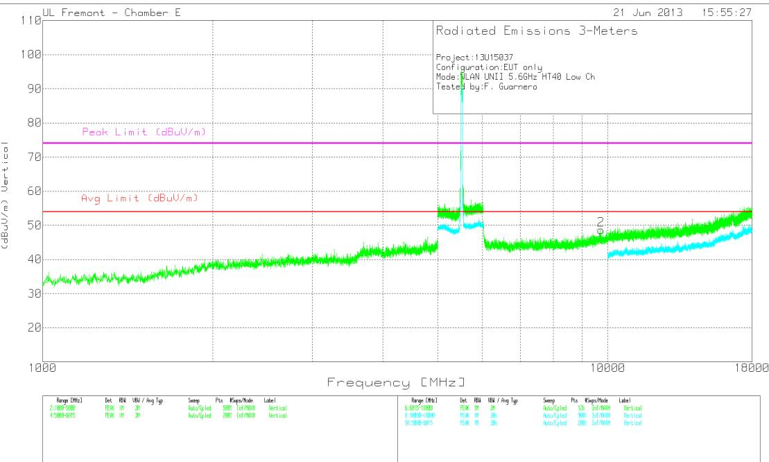
FCC Part15C All 5GHz UNII and DTS Spurious Emissions with Average Scan.TST 30915 19 Jun 2013
