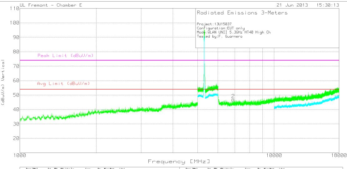
FCC Part15C All 5GHz UNII and DTS Spurious Emissions with Average Scan.TST 38915 19 Jun 2013
