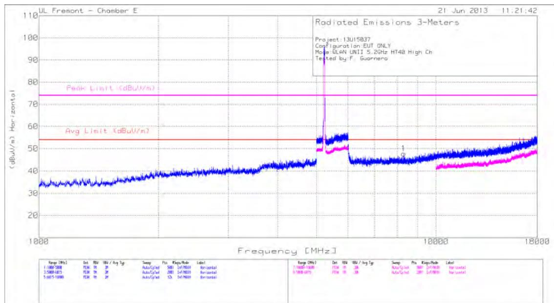
FCC Part15C All 5GHz UNII and DTS Spurious Emissions with Average Scan TSI 38915 19 Jun 2013
