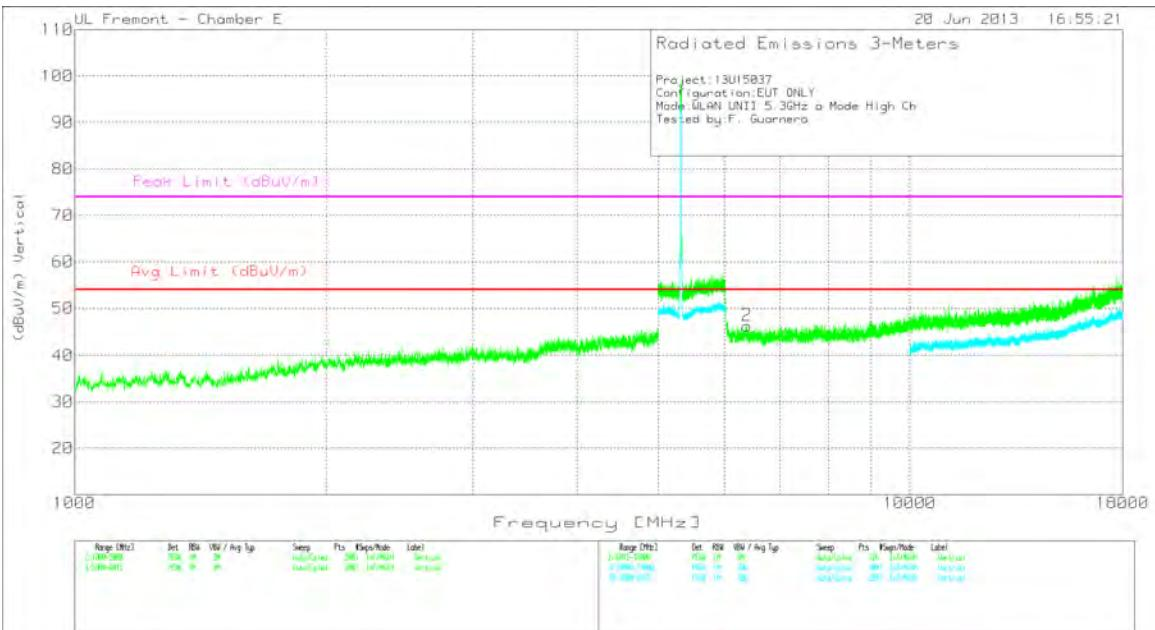
FCC Part 15C All 5GHz UNII and DTS Spurious Emissions with Average Scan-TST 38915 19 Jun 2013
