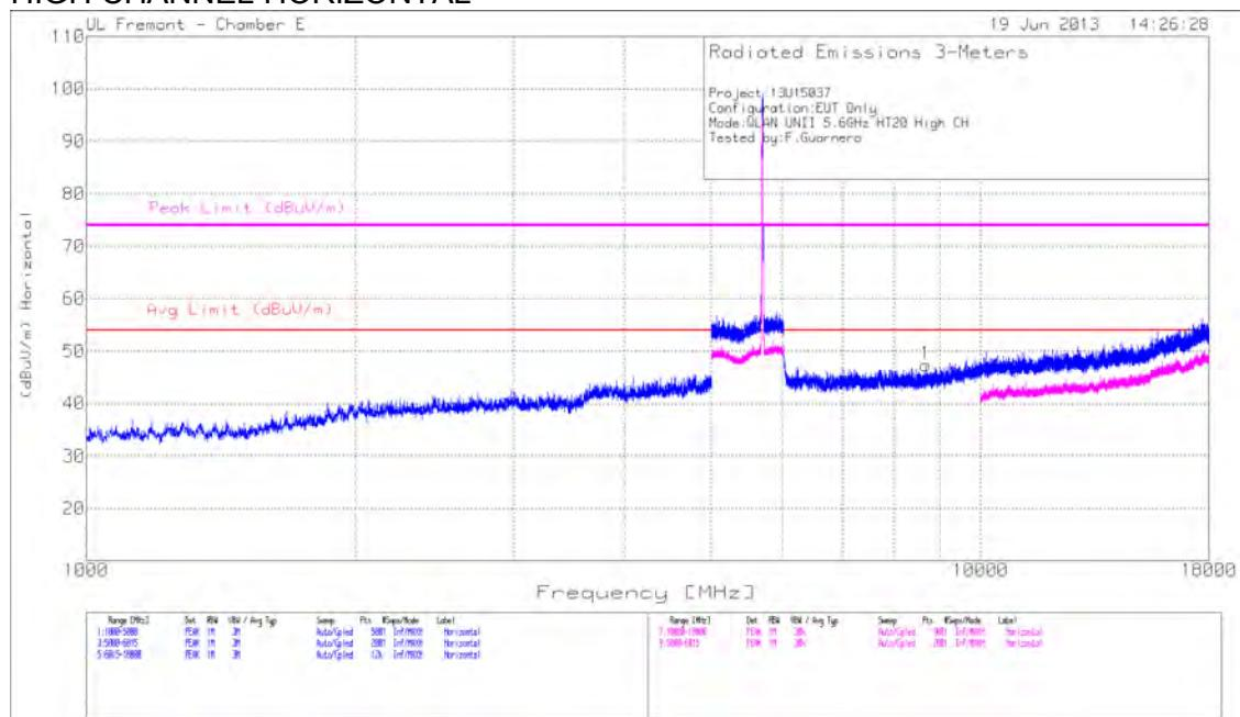
FCC Part15C All 5GHz UNIT and DTS Spurious Emissions with Average Scan TST 30915 19 Jun 2013 Rev 9.5 13 Jun 2013
