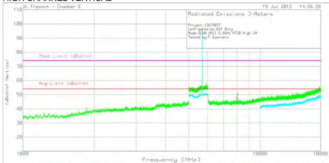
FCC Part15C All 5GHz UNII and DTS Spurious Emissions with Average Scan TST 30915 19 Jun 2013
