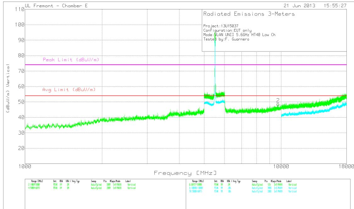
FCC Part15C All 5GHz UNII and DTS Spurious Emissions with Average Scan.TST 30915 19 Jun 2013
