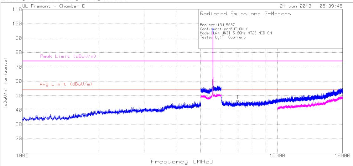
FCC Part15C All 5GHz UNII and DTS Spurious Emissions with Average Scan,TST 30915 19 Jun 2013
