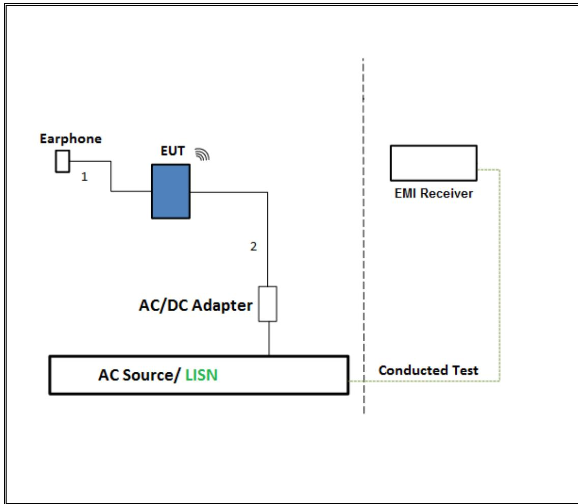
**TEST SETUP- AC LINE CONDUCTED: LAPTOP CONFIGURATION**
