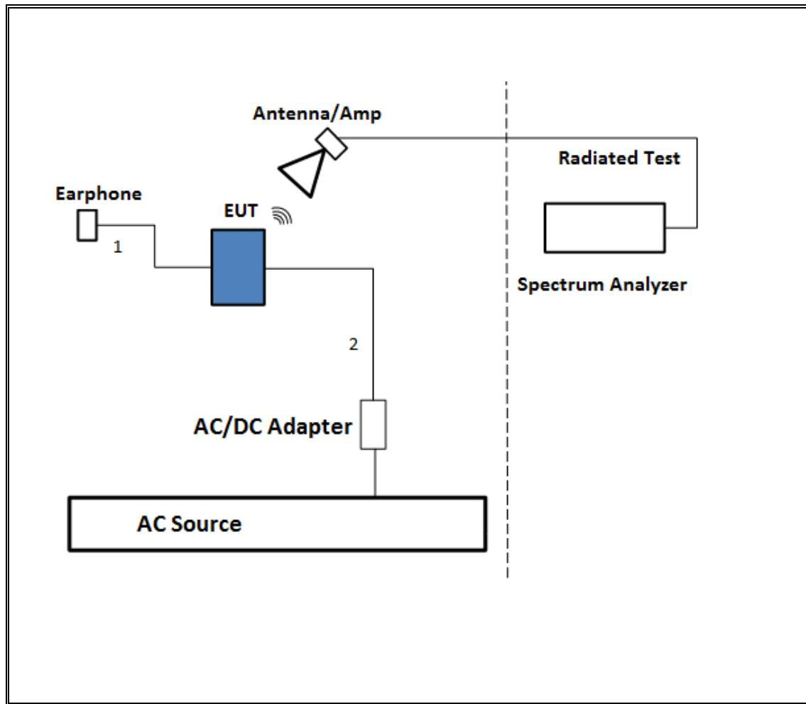
**TEST SETUP- AC LINE CONDUCTED: AC/DC ADAPTER**
