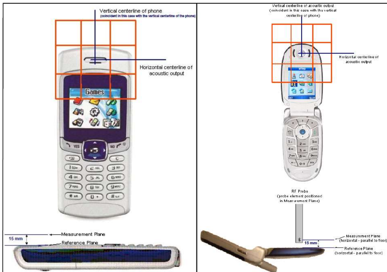
Figure 1 - WD reference and plane for RF emission measurements
