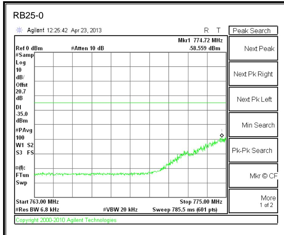
**LTE 16QAM 784.5MHz Band 13, 763-775MHz (5MHz Bandwidth)**
