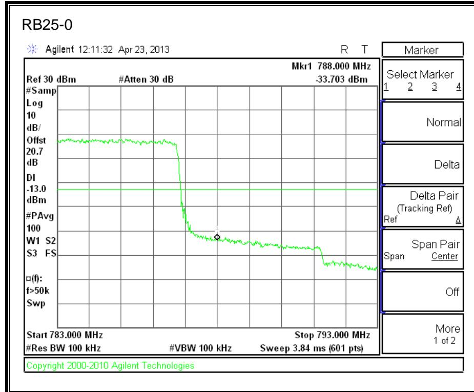
**LTE 16QAM 784.5MHz Band 13, 783 - 793MHz (5MHz Bandwidth)**
