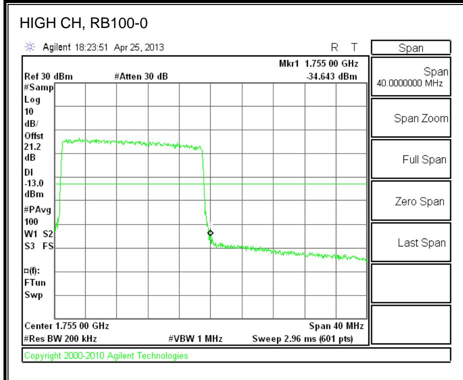
**LTE 16QAM Band 4 (20.0 MHz BAND WIDTH)**
