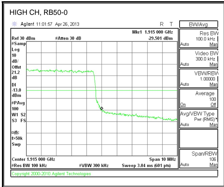
**LTE 16QAM Band 25 (10.0 MHz BAND WIDTH)**
