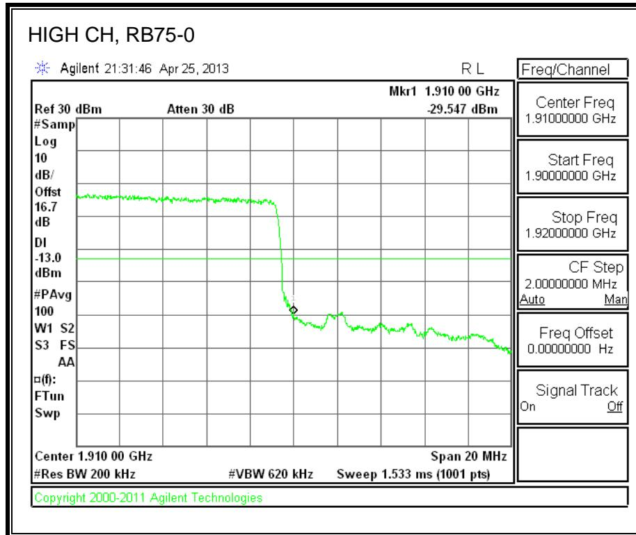
**LTE 16QAM Band 2 (15.0 MHz BAND WIDTH)**
