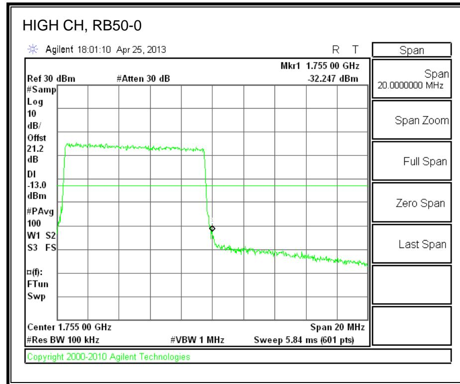
**LTE QPSK Band 4 (15.0 MHz BAND WIDTH)**
