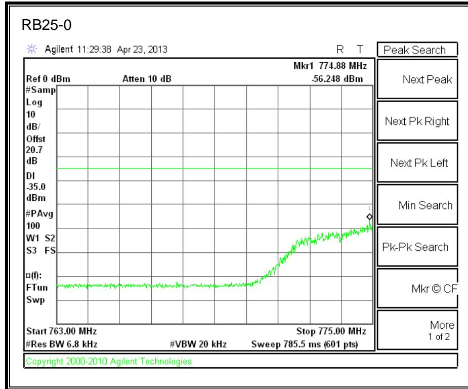
**LTE 16QAM 782MHz Band 13, 763-775MHz (5MHz Bandwidth)**
