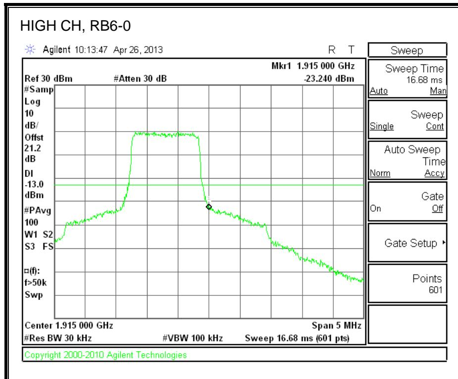
**LTE 16QAM Band 25 (1.4 MHz BAND WIDTH)**
