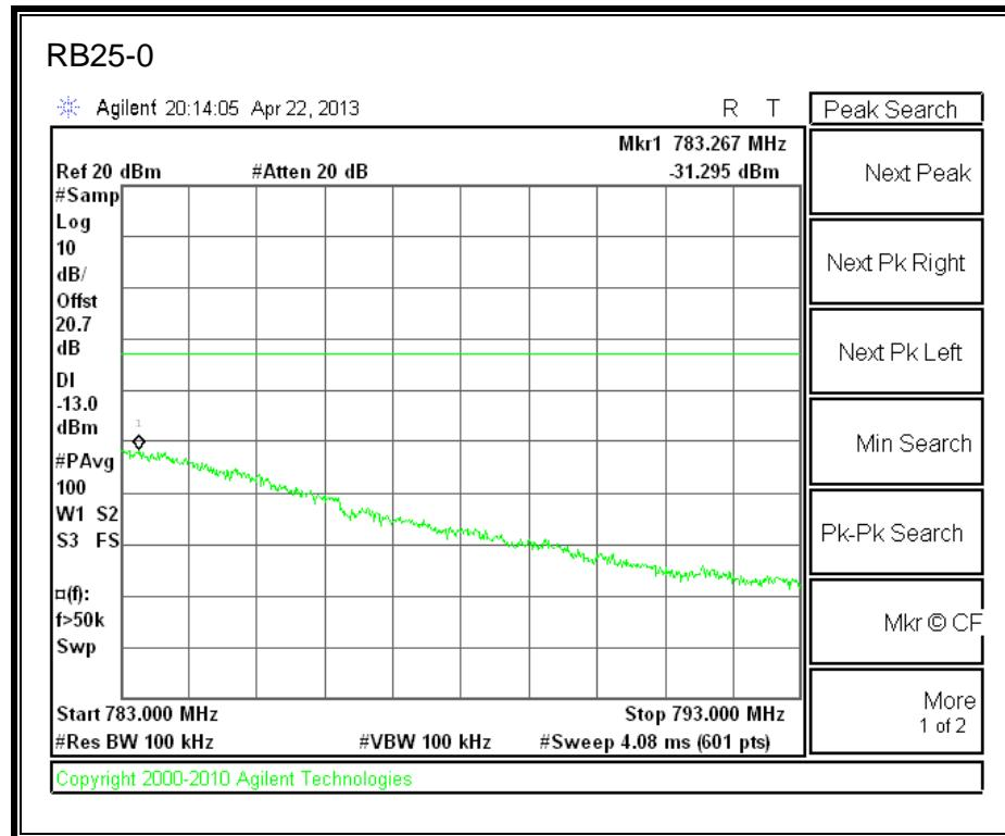
**LTE QPSK 779.5MHz Band 13, 763 - 775MHz (5MHz Bandwidth)**
