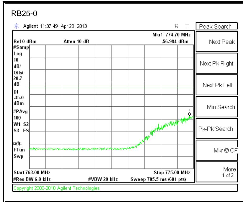
**LTE QPSK 782MHz Band 13, 793 - 805MHz (5MHz Bandwidth)**
