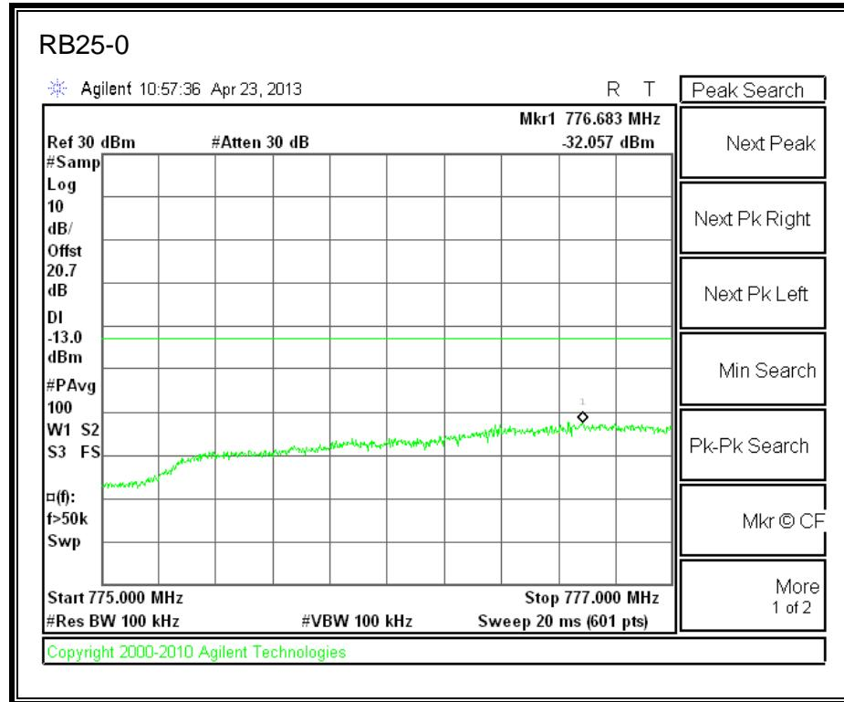
**LTE 16QAM 782MHz Band 13, 775 - 777MHz (5MHz Bandwidth)**
