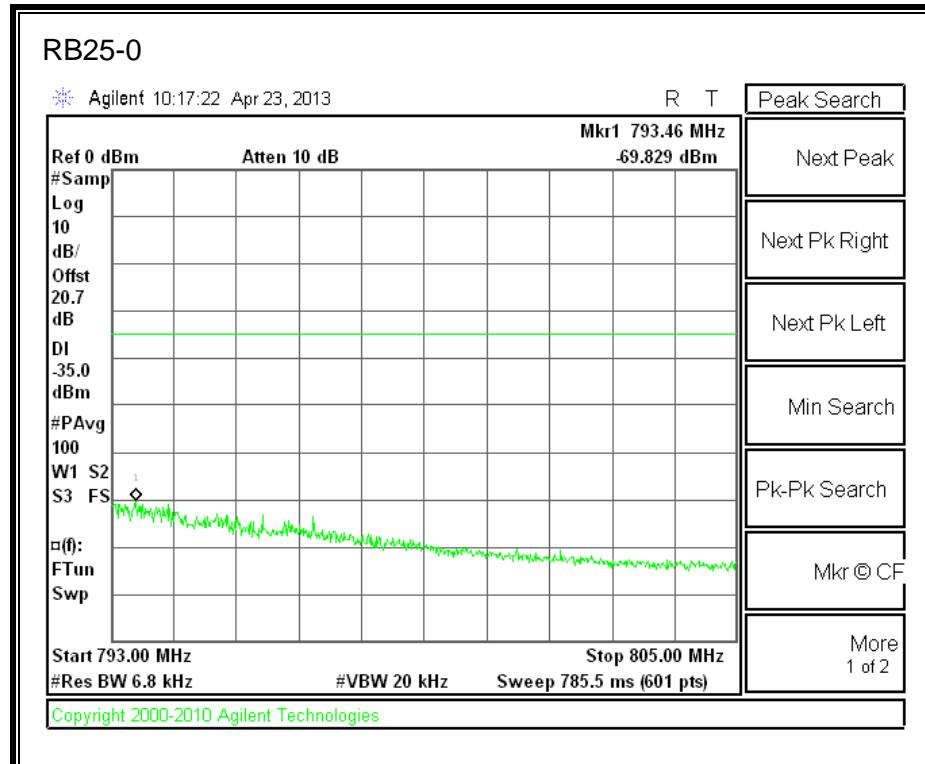
**LTE QPSK 782MHz Band 13, 775 - 777MHz (5MHz Bandwidth)**
