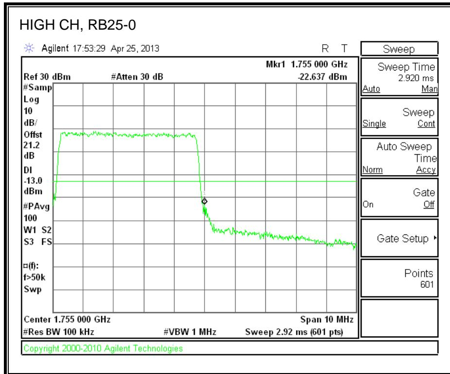
**LTE 16QAM Band 4 (5.0 MHz BAND WIDTH)**
