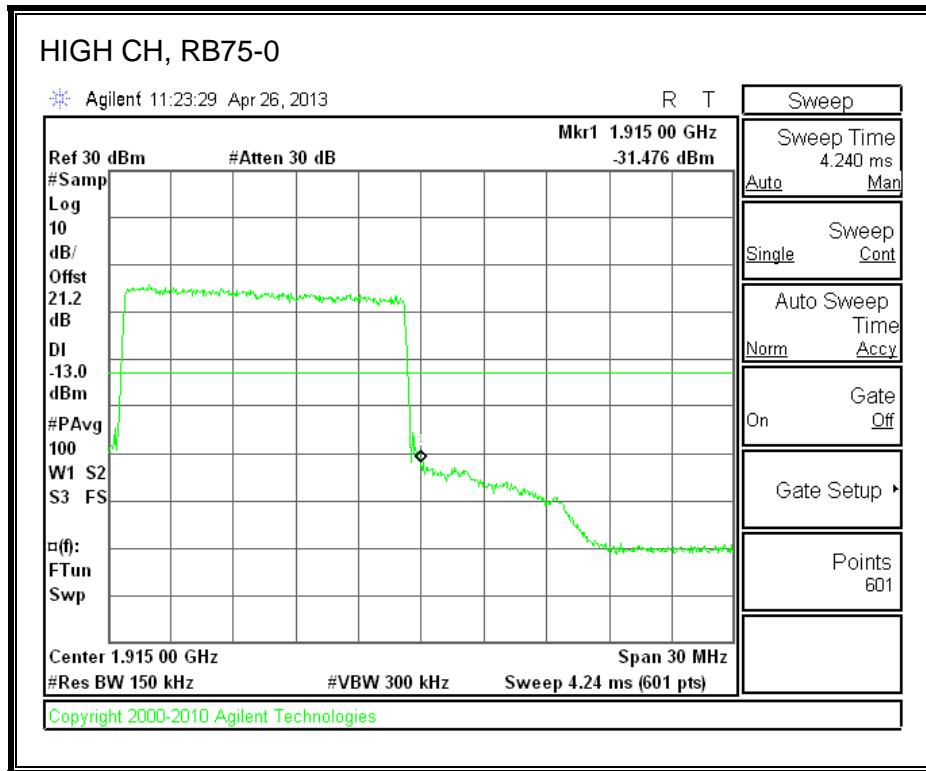
**LTE QPSK Band 25 (20.0 MHz BAND WIDTH)**
