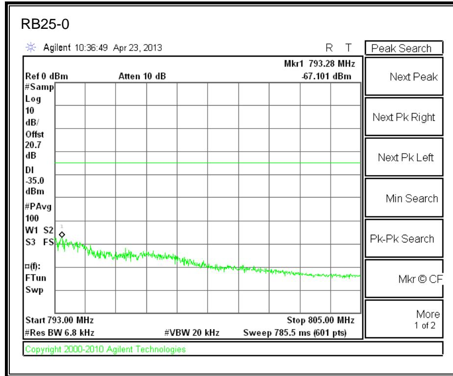
**LTE 16QAM 779.5MHz Band 13, 793 - 805MHz (5MHz Bandwidth)**
