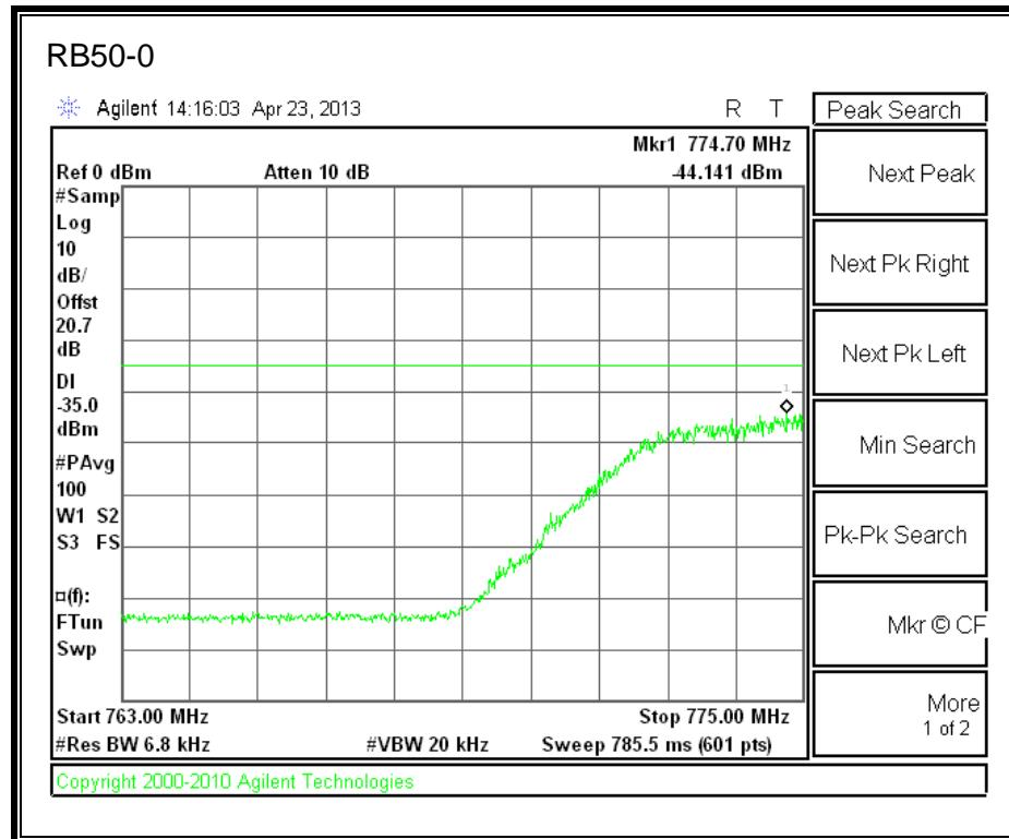
**LTE 16QAM 782MHz Band 13, 763 - 775MHz (10MHz Bandwidth)**
