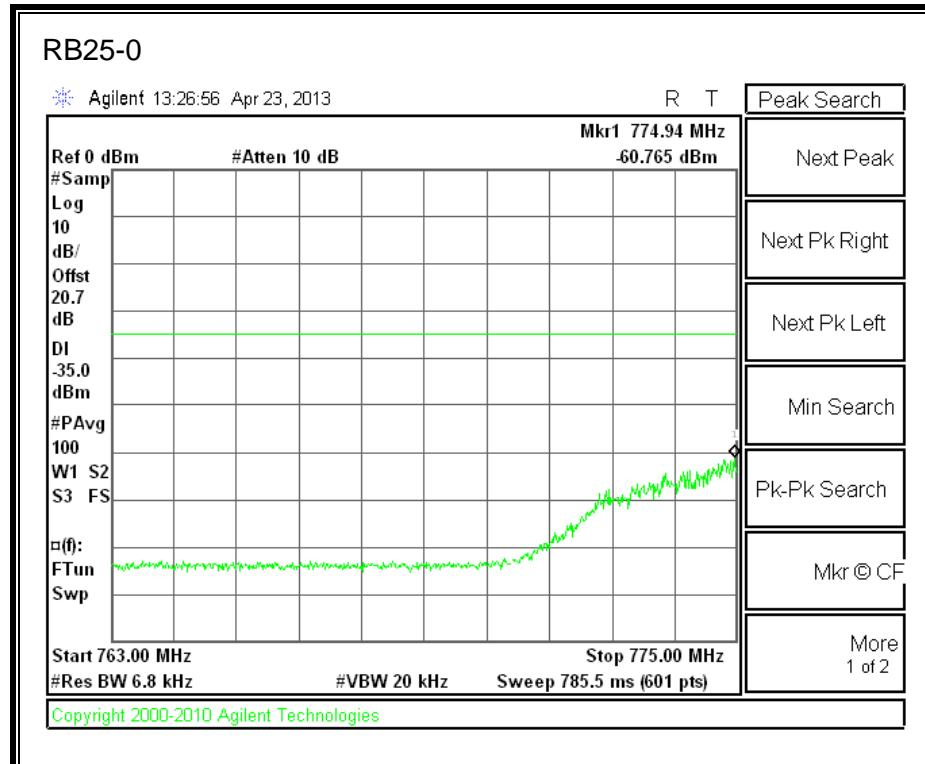
**LTE QPSK 784.5MHz Band 13, 793 - 805MHz (5MHz Bandwidth)**
