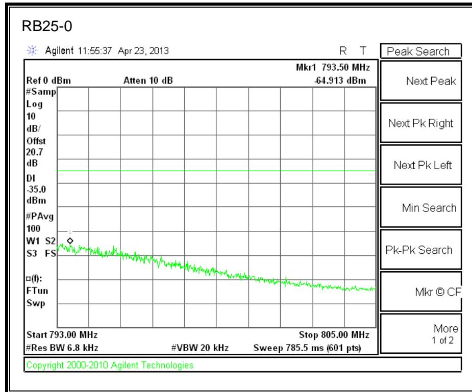
LTE QPSK 784.5 MHz Band 13, 775 - 777MHz (5MHz Bandwidth)
