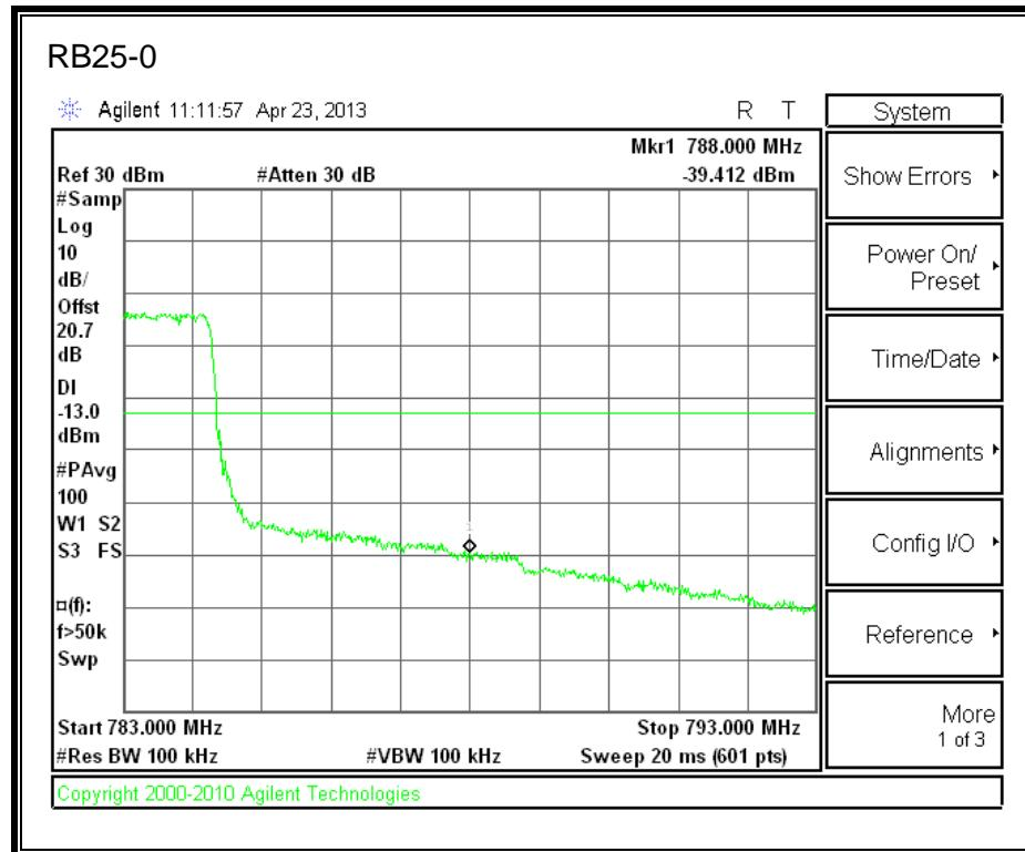
**LTE QPSK 782MHz Band 13, 763 - 775MHz (5MHz Bandwidth)**
