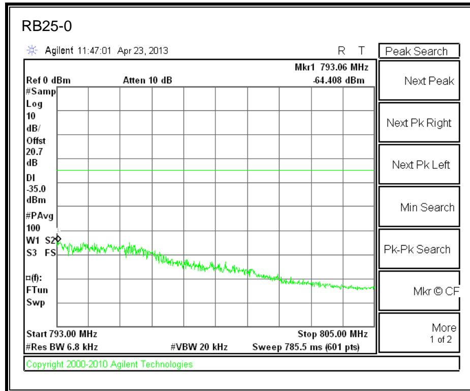
**LTE 16QAM 7825MHz Band 13, 793 - 805MHz (5MHz Bandwidth)**
