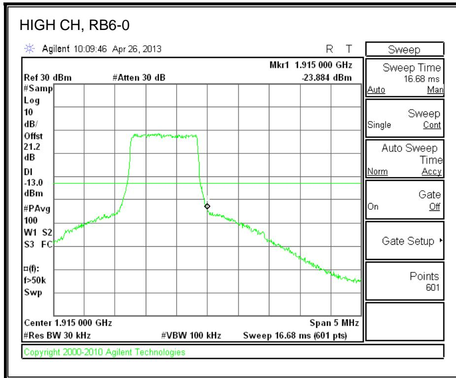
**LTE QPSK Band 25 (3.0 MHz BAND WIDTH)**
