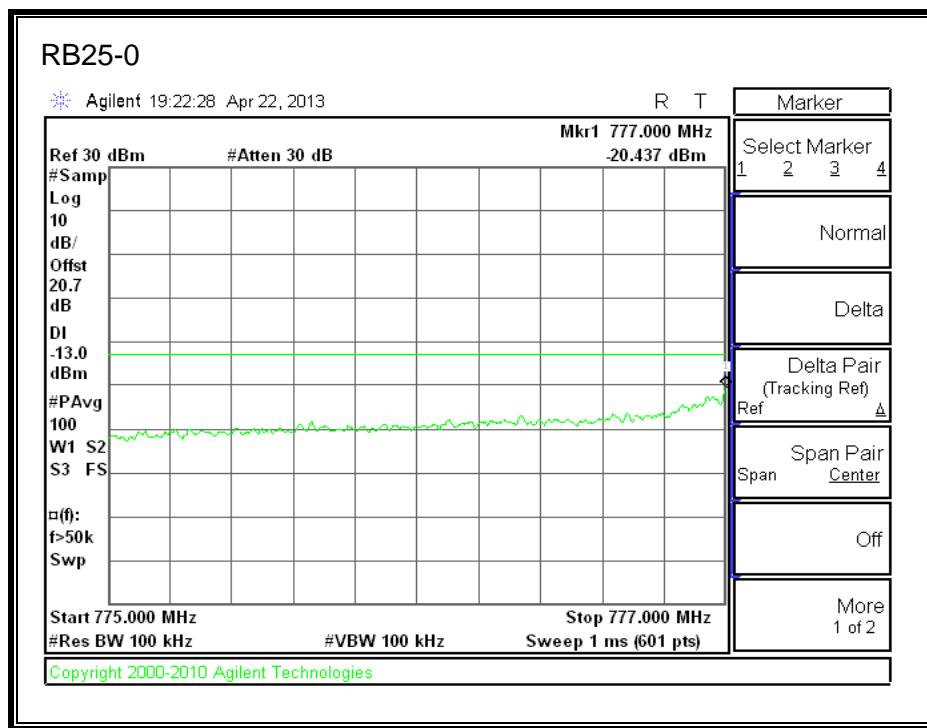
**LTE 16QAM 779.5MHz Band 13, 775 - 777MHz (5MHz Bandwidth)**
