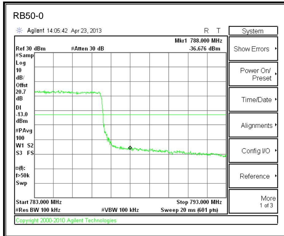
**LTE QPSK 782MHz Band 13, 763 - 775MHz (10MHz Bandwidth)**
