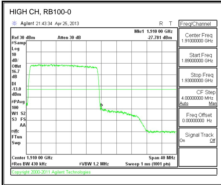
**LTE 16QAM Band 2 (20.0 MHz BAND WIDTH)**
