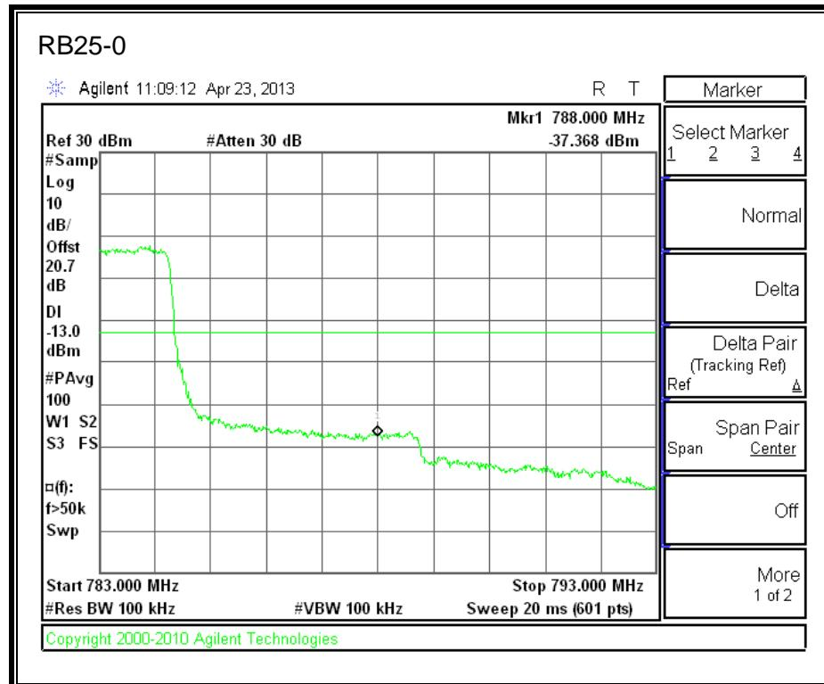
**LTE 16QAM 782MHz Band 13, 783 - 793MHz (5MHz Bandwidth)**
