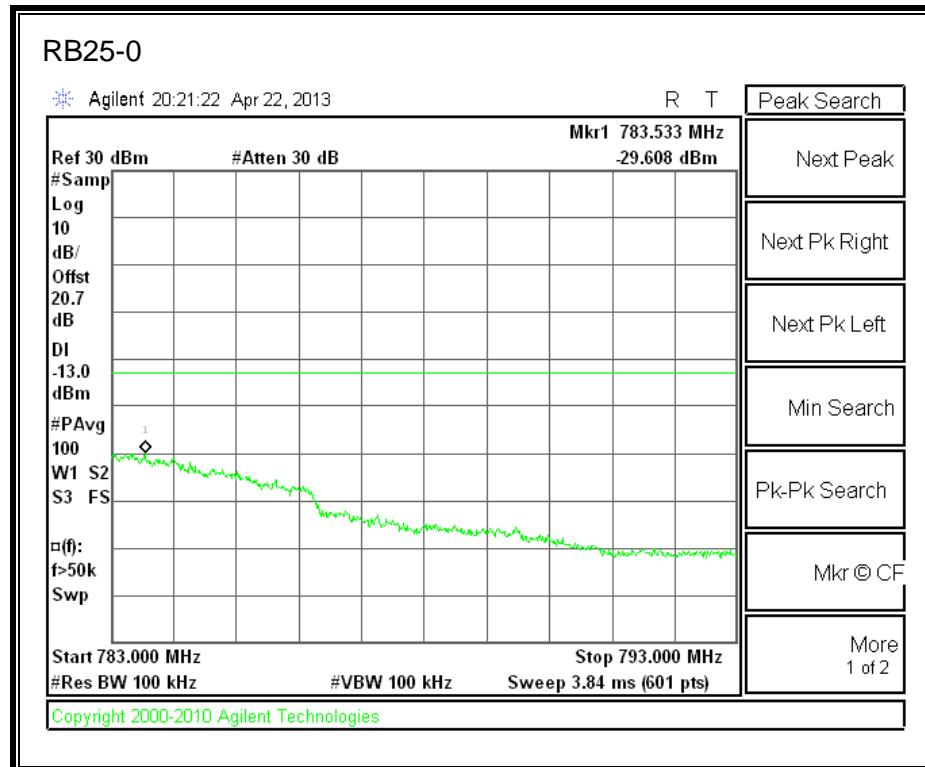
**LTE 16QAM 779.5MHz Band 13, 783 - 793MHz (5MHz Bandwidth)**
