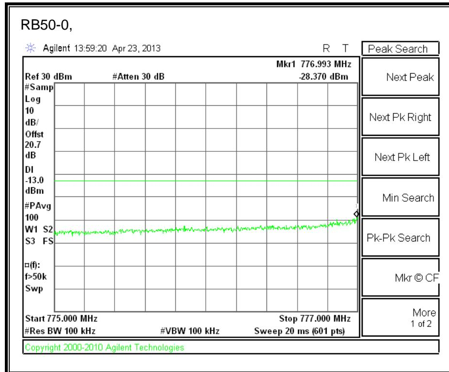
**LTE QPSK 782MHz Band 13, 783 - 793MHz (10MHz Bandwidth)**
