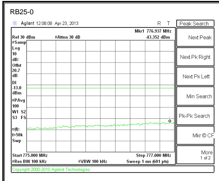
**LTE QPSK 784.5MHz Band 13, 783 - 793MHz (5MHz Bandwidth)**
