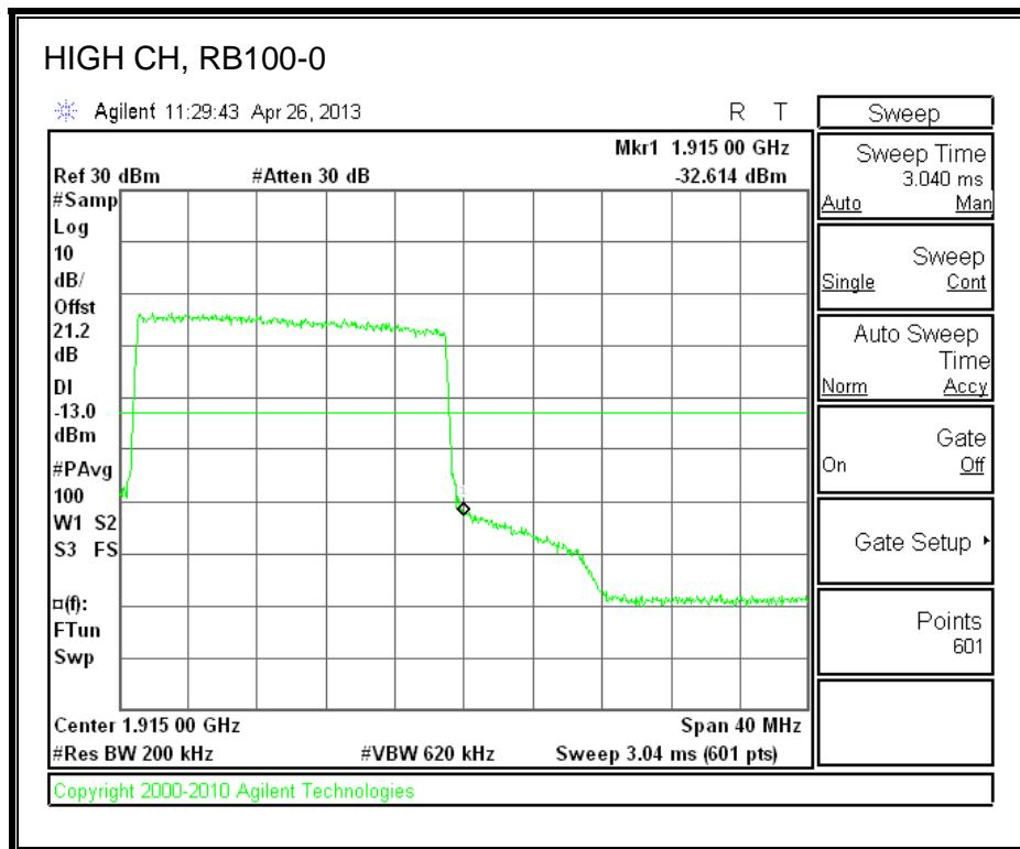
**LTE 16QAM Band 25 (20.0 MHz BAND WIDTH)**
