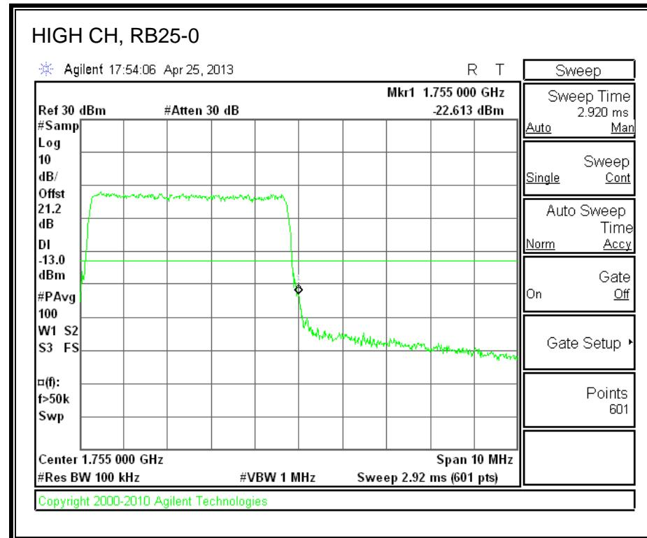
**LTE QPSK Band 4 (10.0 MHz BAND WIDTH)**
