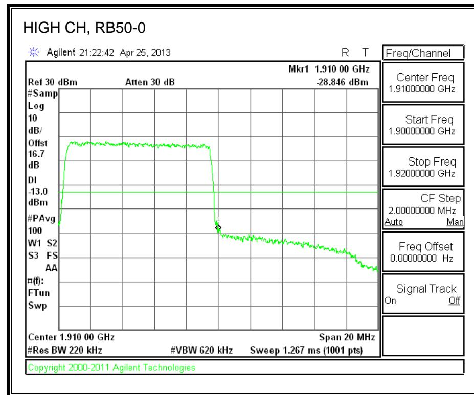
**LTE QPSK Band 2 (15.0 MHz BAND WIDTH )**
