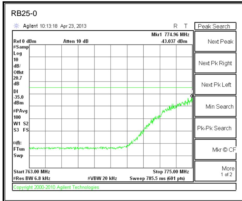
**LTE QPSK 779.5MHz Band 13, 793 - 805MHz (5MHz Bandwidth)**
