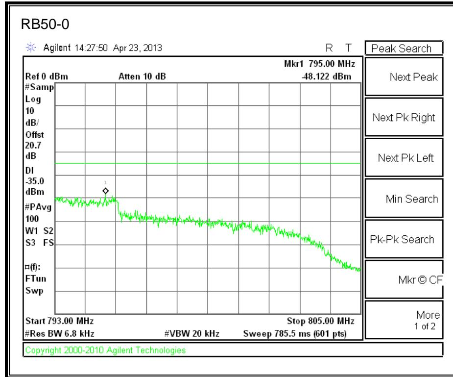
**LTE 16QAM Band 13, 793 - 805MHz (10MHz Bandwidth)**
