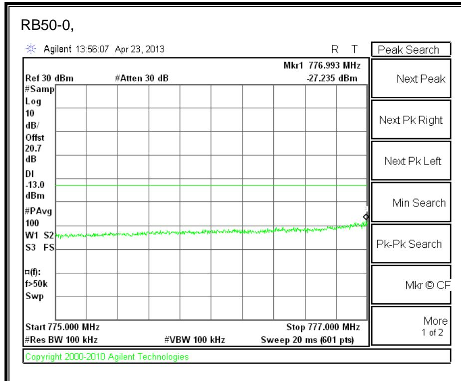
**LTE 16QAM Band 13, 775 - 777MHz (10MHz Bandwidth)**
