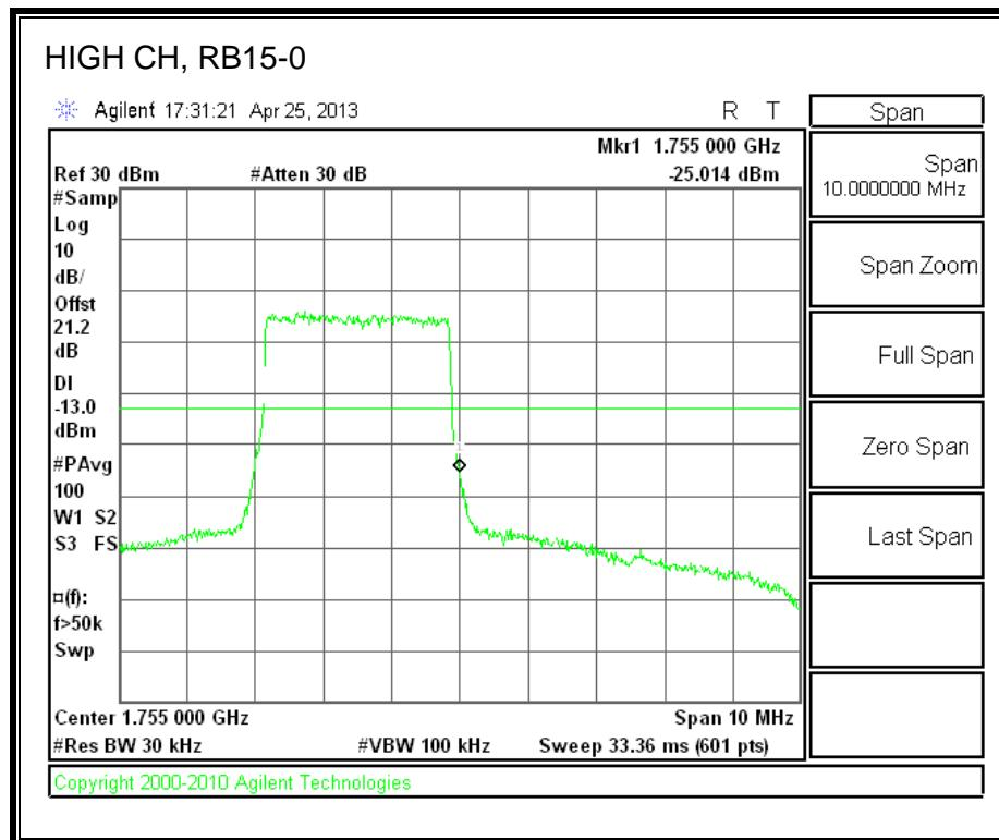
**LTE 16QAM Band 4 (3.0 MHz BAND WIDTH)**
