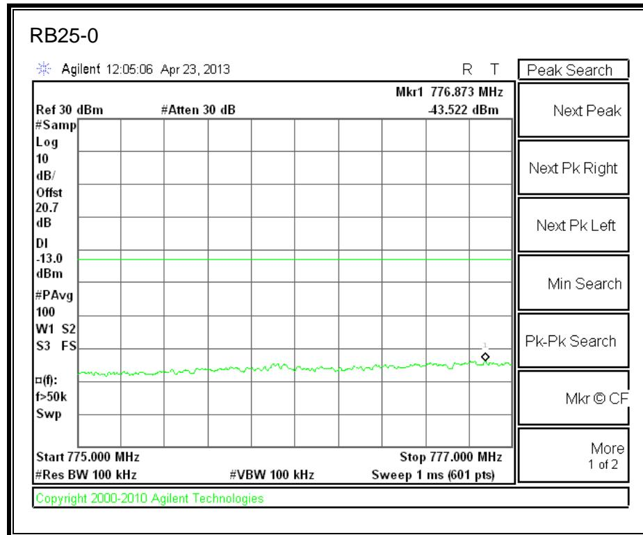
**LTE 16QAM 784.5MHz Band 13, 775 - 777MHz (5MHz Bandwidth)**
