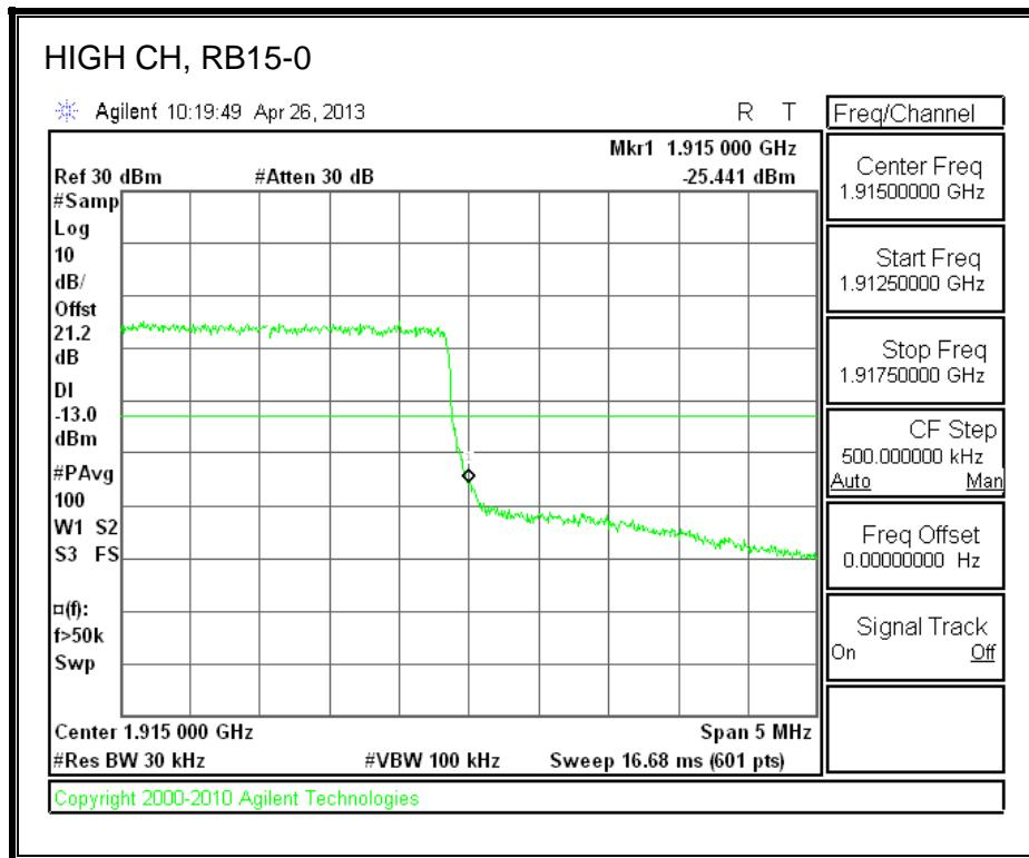
**LTE QPSK Band 25 (5.0 MHz BAND WIDTH)**
