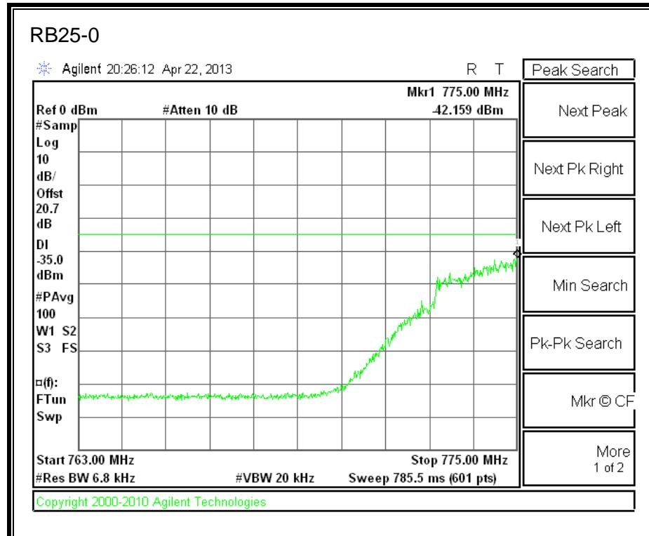
**LTE 16QAM 779.5MHz Band 13, 763-775MHz (5MHz Bandwidth)**
