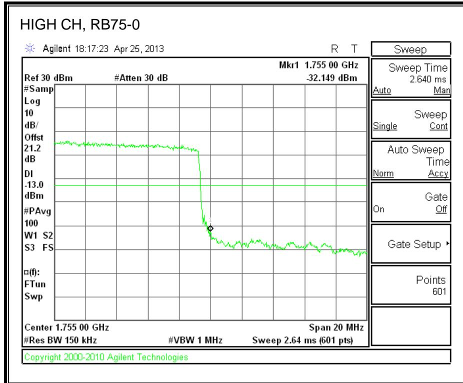
**LTE 16QAM Band 4 (15.0 MHz BAND WIDTH)**
