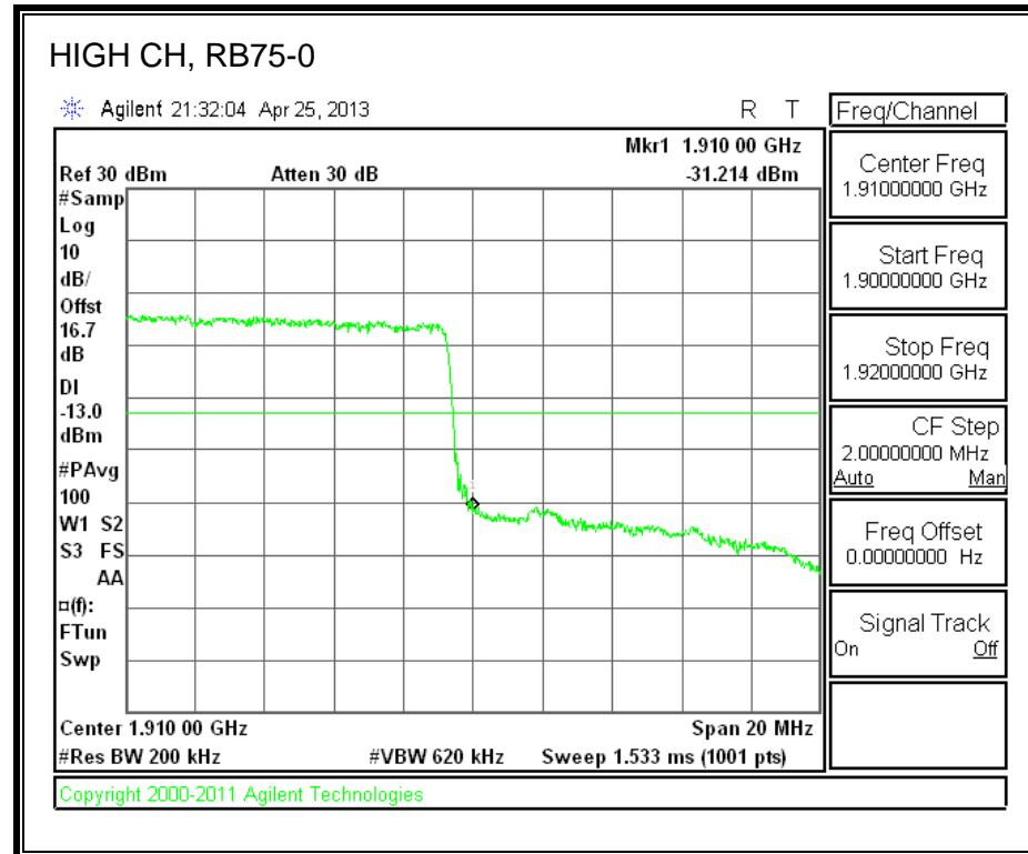
**LTE QPSK Band 2 (20.0 MHz BAND WIDTH)**
