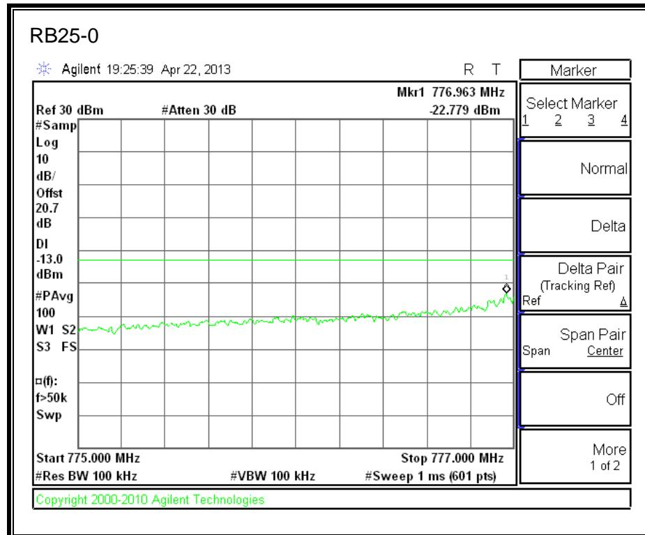
**LTE QPSK 779.5MHz Band 13, 783 - 793MHz (5MHz Bandwidth)**
