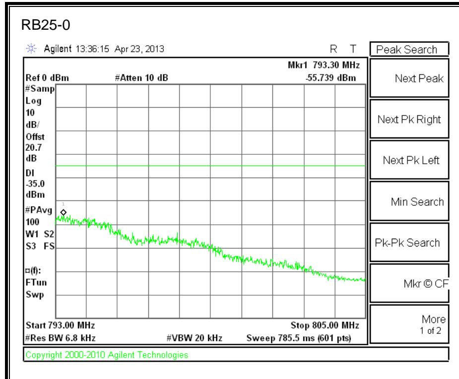
**LTE 16QAM 784.5MHz Band 13, 793 - 805MHz (5MHz Bandwidth)**
