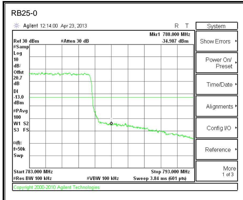
**LTE QPSK 784.5MHz Band 13, 763 - 775MHz (5MHz Bandwidth)**
