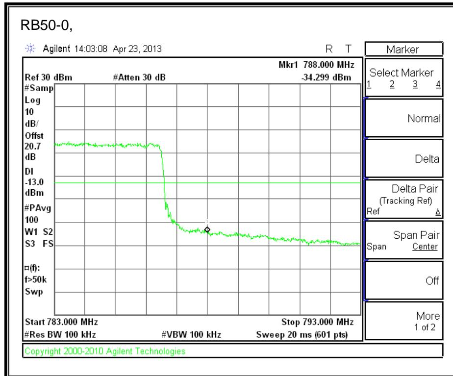
**LTE 16QAM Band 13, 782MHz 783 - 793MHz (10MHz Bandwidth)**
