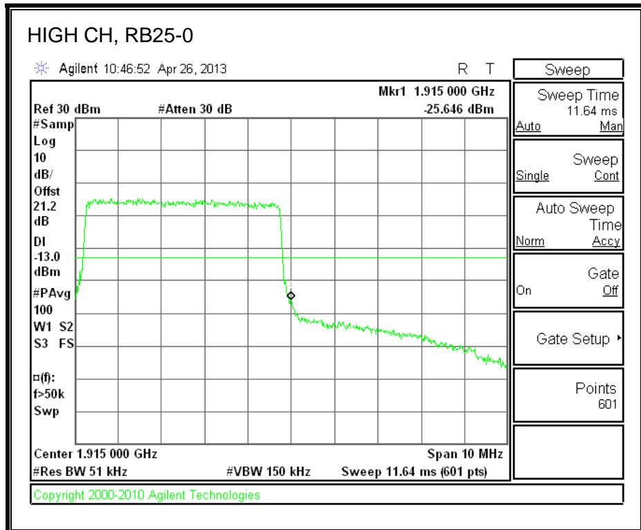
**LTE QPSK Band 25 (10.0 MHz BAND WIDTH)**
