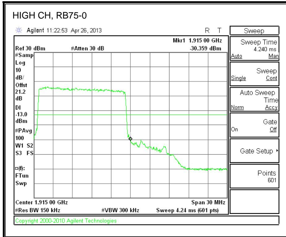
**LTE 16QAM Band 25(15.0 MHz BAND WIDTH)**
