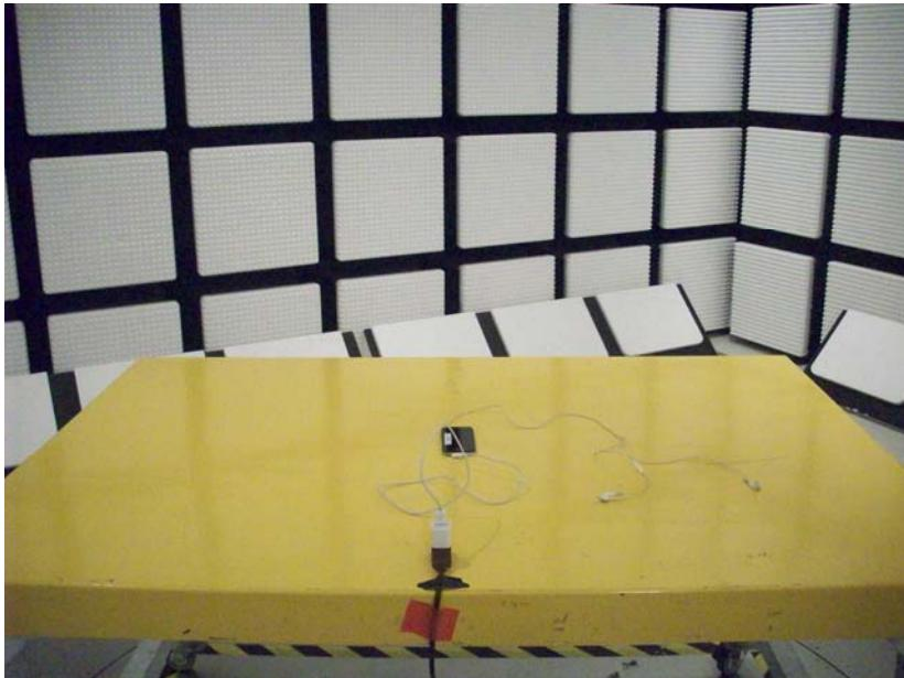
**RADIATED RF MEASUREMENT SETUP FOR PORTABLE CONFIGURATION**
