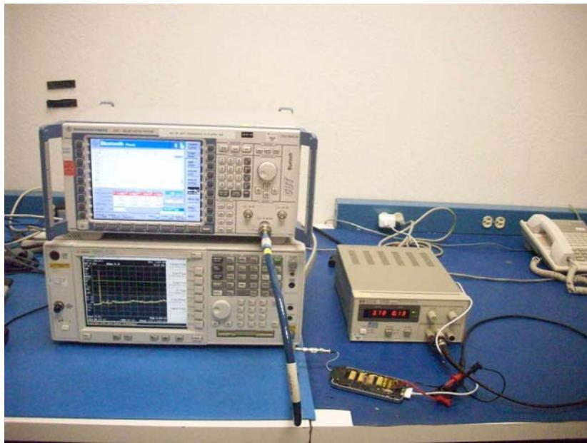
**RADIATED RF MEASUREMENT SETUP**
