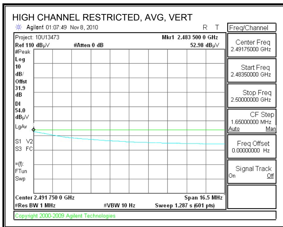
**HARMONICS AND SPURIOUS EMISSIONS****High Frequency Measurement
