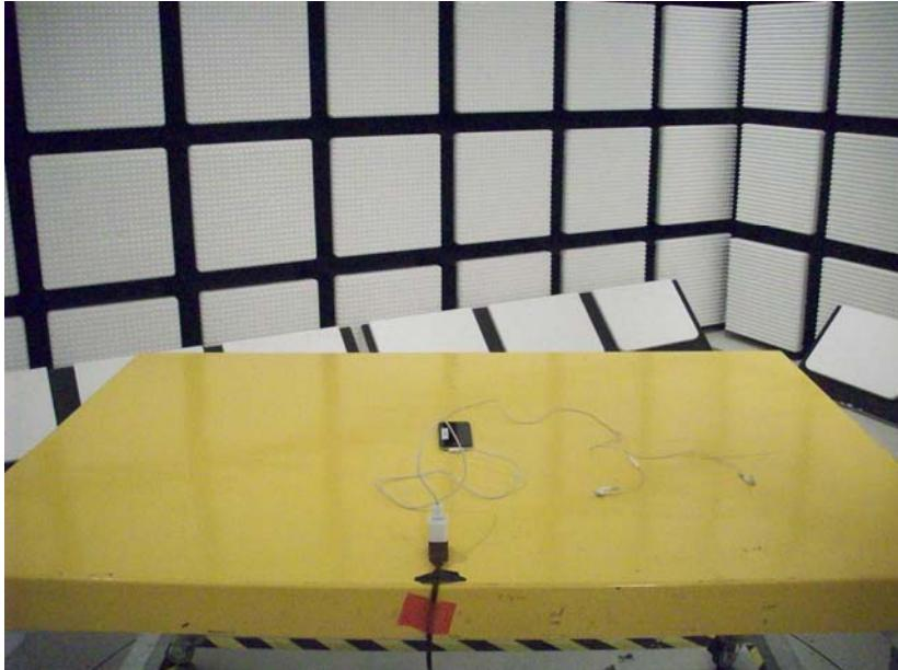
**RADIATED RF MEASUREMENT SETUP FOR PORTABLE CONFIGURATION**
