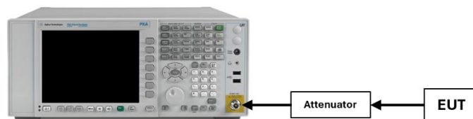
Figure 7-4. Test Instrument & Measurement Setup
