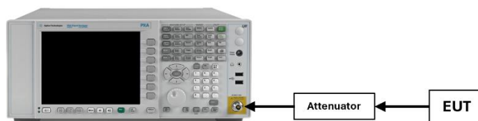
Figure 7-5. Test Instrument & Measurement Setup
