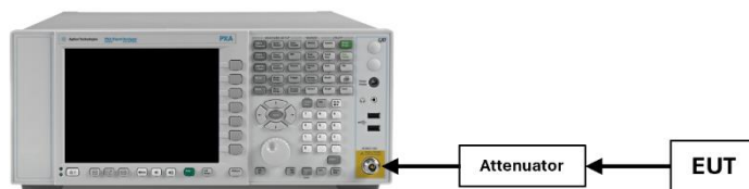
Figure 7-3. Test Instrument & Measurement Setup
