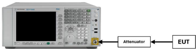
Figure 7-1. Test Instrument & Measurement Setup
