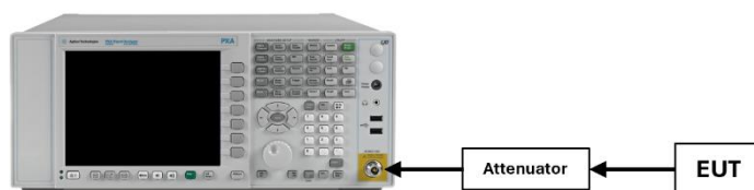
Figure 7-3. Test Instrument & Measurement Setup
