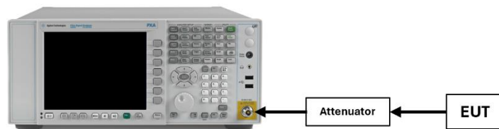
Figure 7-5. Test Instrument & Measurement Setup
