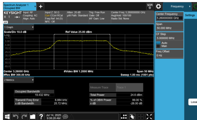
Plot 7-4. 26dB BW & 99% OBW (20MHz BW 802.11n – Ch. 52, MCS0)
