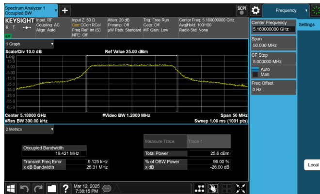
Plot 7-1. 26dB BW & 99% OBW (20MHz BW 802.11n – Ch. 36, MCS0)
