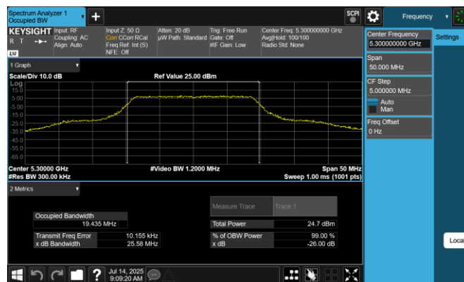
Plot 7-5. 26dB BW & 99% OBW (20MHz BW 802.11n – Ch. 60, MCS0)
