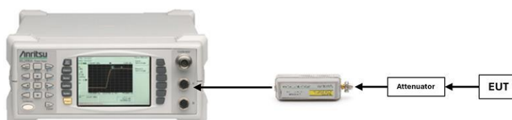
Figure 7-3. Test Instrument & Measurement Setup
