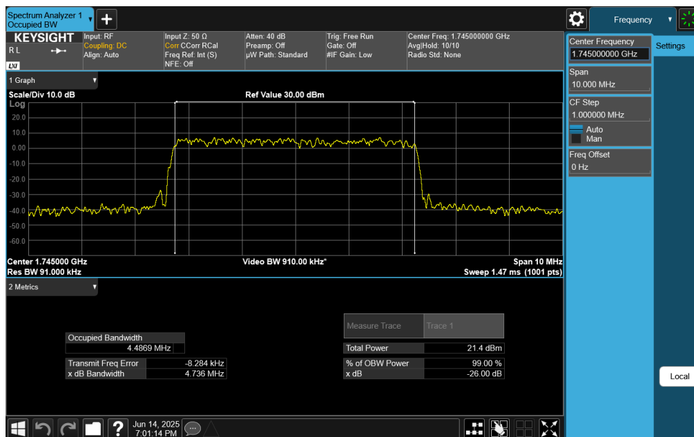
Plot 7-36. Occupied Bandwidth Plot (NR Band n66 - 5.0MHz CP-OFDM 64QAM - Full RB)
