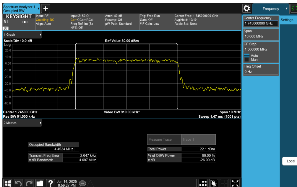
Plot 7-34. Occupied Bandwidth Plot (NR Band n66 - 5.0MHz CP-OFDM QPSK - Full RB)
