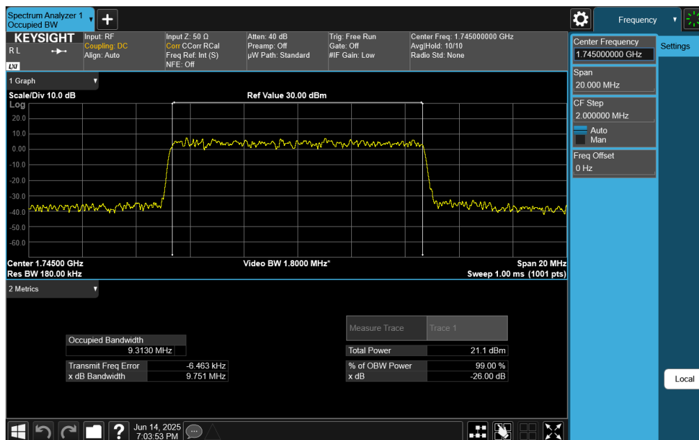
Plot 7-40. Occupied Bandwidth Plot (NR Band n66 - 10.0MHz CP-OFDM 64QAM - Full RB)
