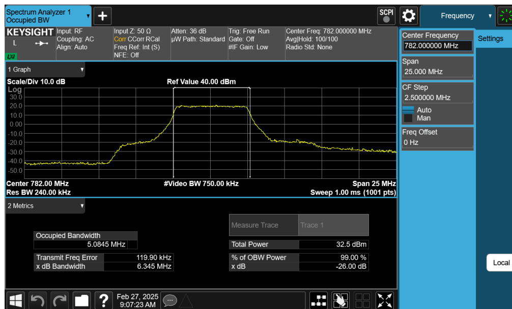
Plot 7-32. Occupied Bandwidth Plot (LTE Band 13 - 10MHz 16-QAM - Full RB)
