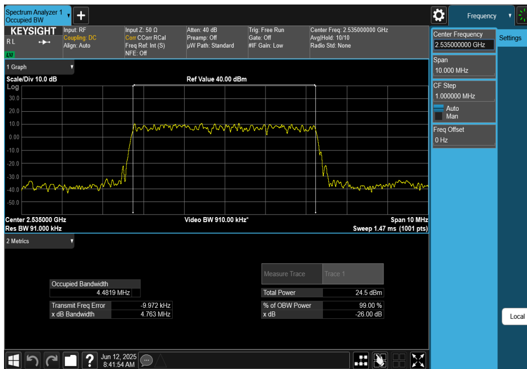
Plot 7-17. Occupied Bandwidth Plot (NR Band n7 - 5MHz DFT-s-OFDM \pi/2 BPSK - Full RB)
