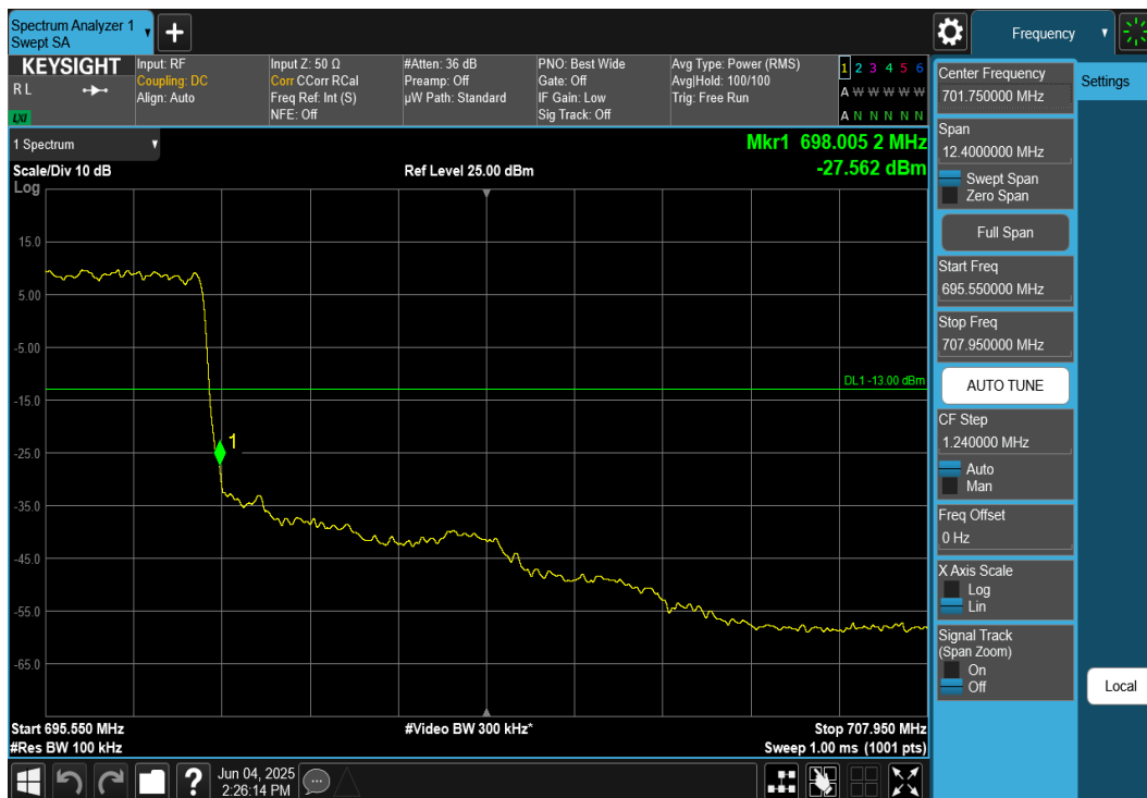
Plot 7-229. Upper Band Edge Plot (NR Band n71 – 5MHz DFT-S-OFDM \pi/2 BPSK - Full RB)
