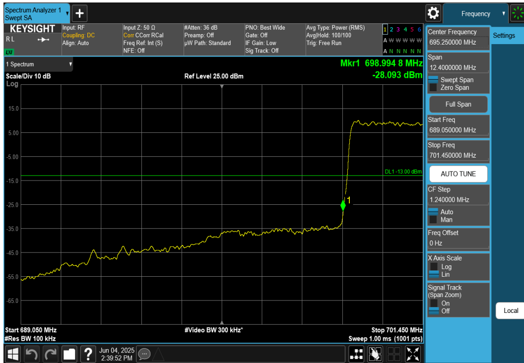
Plot 7-236. Lower Band Edge Plot (NR Band n12 – 5MHz DFT-S-OFDM \pi/2 BPSK - Full RB)
