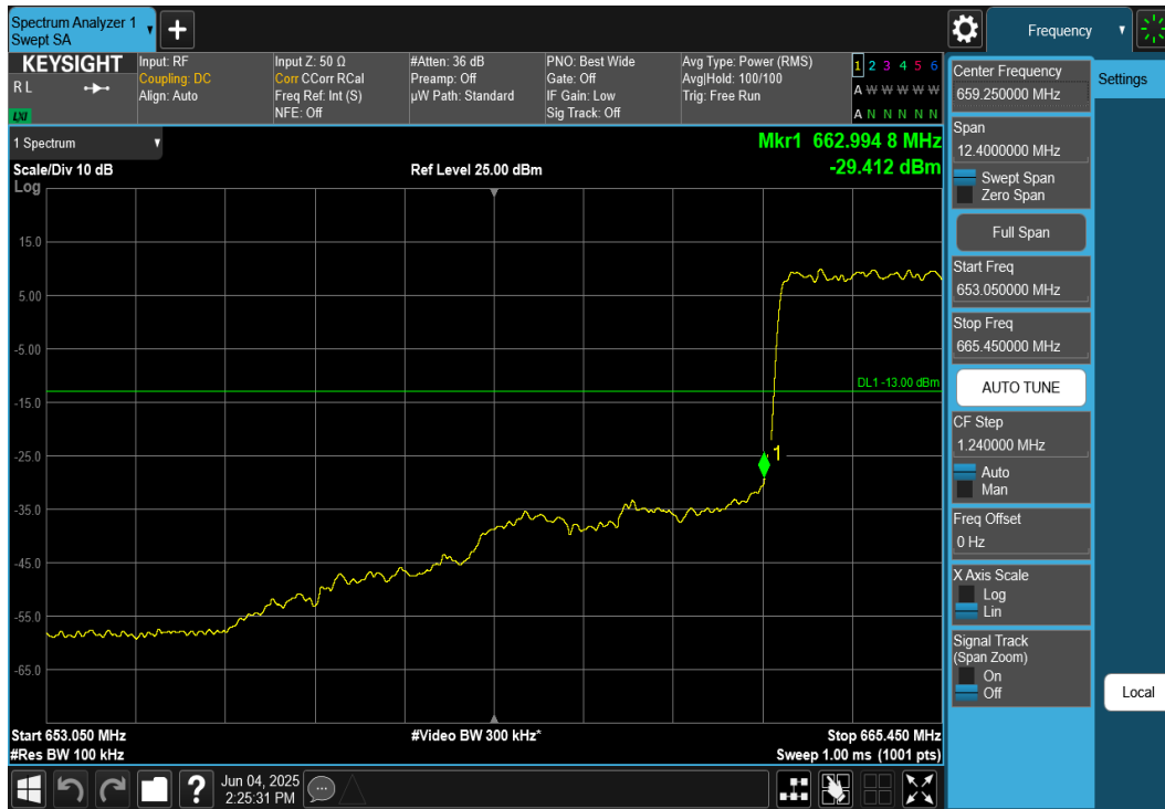
Plot 7-228. Lower Band Edge Plot (NR Band n71 – 5MHz DFT-S-OFDM \pi/2 BPSK - Full RB)
