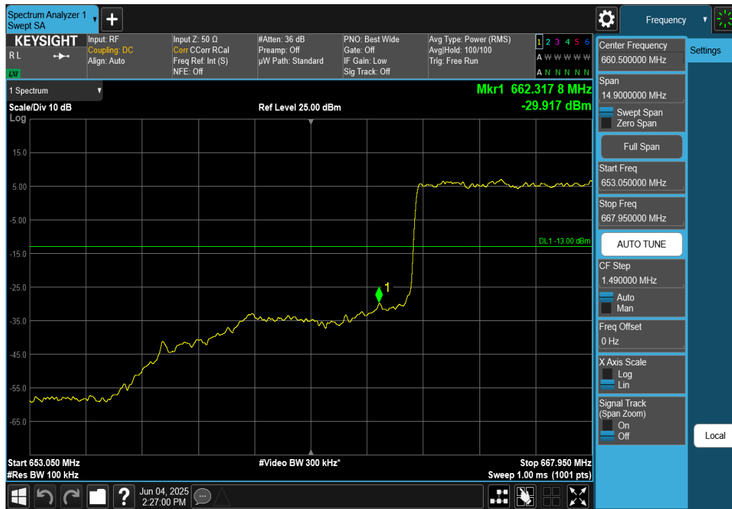
Plot 7-230. Lower Band Edge Plot (NR Band n71 – 10MHz DFT-S-OFDM \pi/2 BPSK - Full RB)
