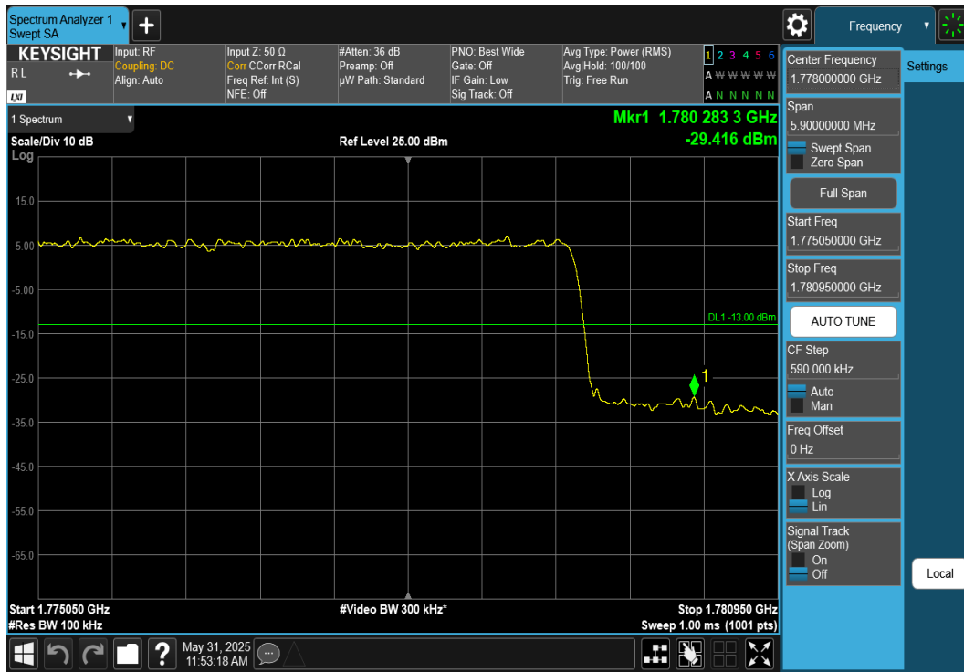
Plot 7-218. Upper Band Edge Plot (NR Band n66 – 10MHz DFT-S-OFDM \pi/2 BPSK - Full RB)
