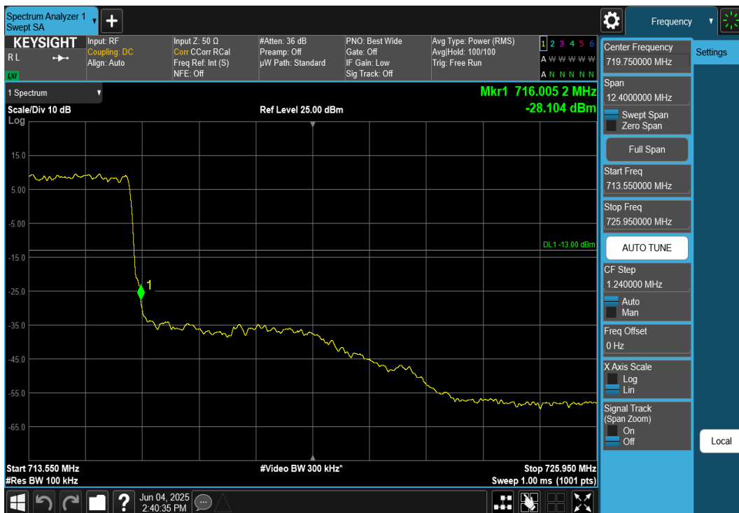
Plot 7-237. Upper Band Edge Plot (NR Band n12 – 5MHz DFT-S-OFDM \pi/2 BPSK - Full RB)
