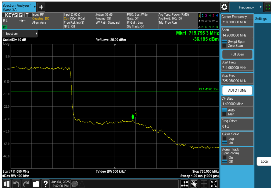
Plot 7-239. Upper Band Edge Plot (NR Band n12 – 10MHz DFT-S-OFDM \pi/2 BPSK - Full RB)
