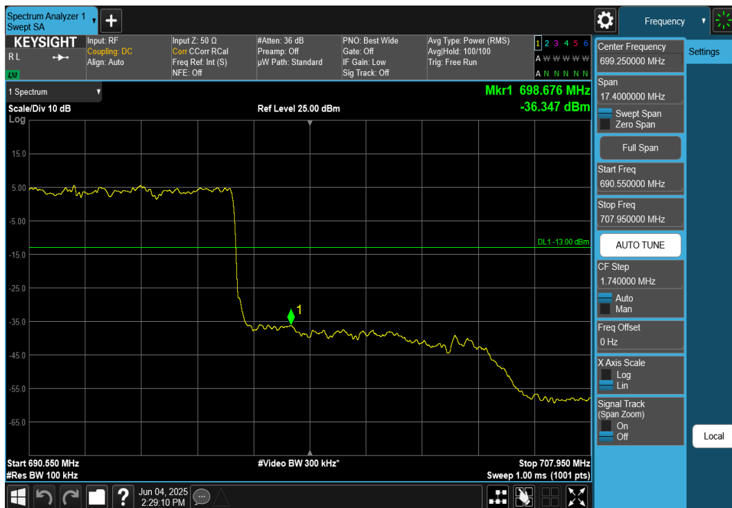
Plot 7-233. Upper Band Edge Plot (NR Band n71 – 15MHz DFT-S-OFDM \pi/2 BPSK - Full RB)
