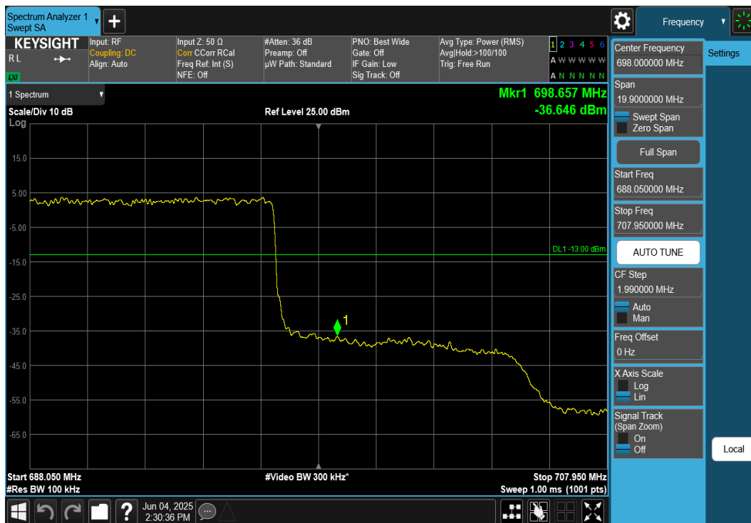
Plot 7-235. Upper Band Edge Plot (NR Band n71 – 20MHz DFT-S-OFDM \pi/2 BPSK - Full RB)
