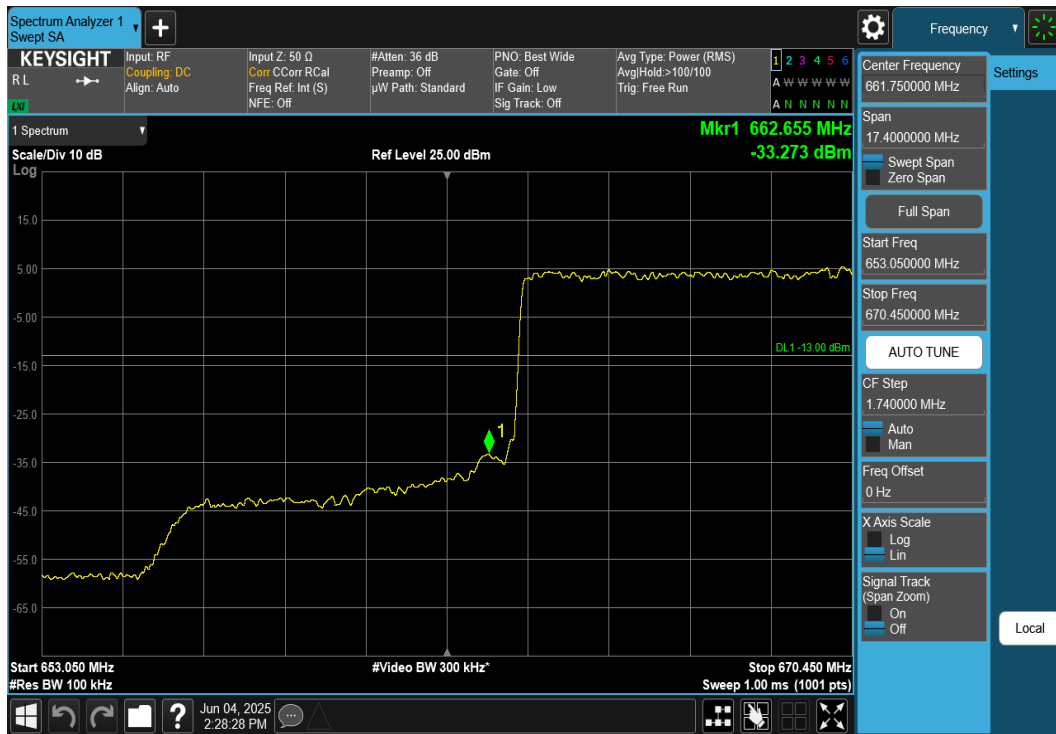
Plot 7-232. Lower Band Edge Plot (NR Band n71 – 15MHz DFT-S-OFDM \pi/2 BPSK - Full RB)
