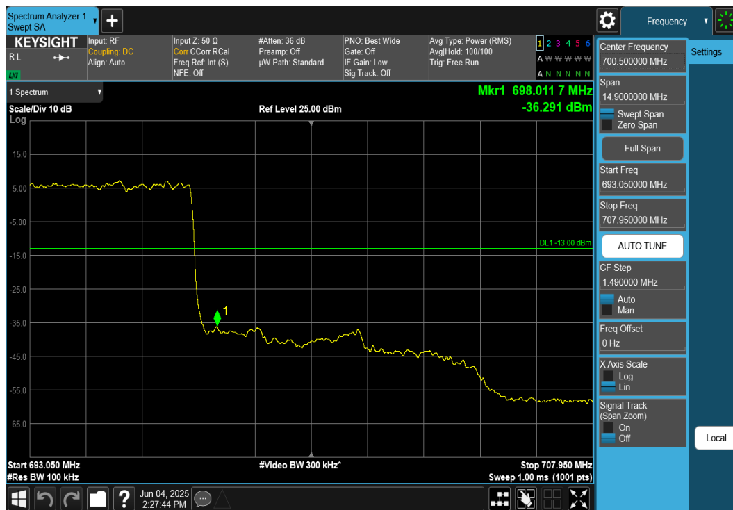
Plot 7-231. Upper Band Edge Plot (NR Band n71 – 10MHz DFT-S-OFDM \pi/2 BPSK - Full RB)
