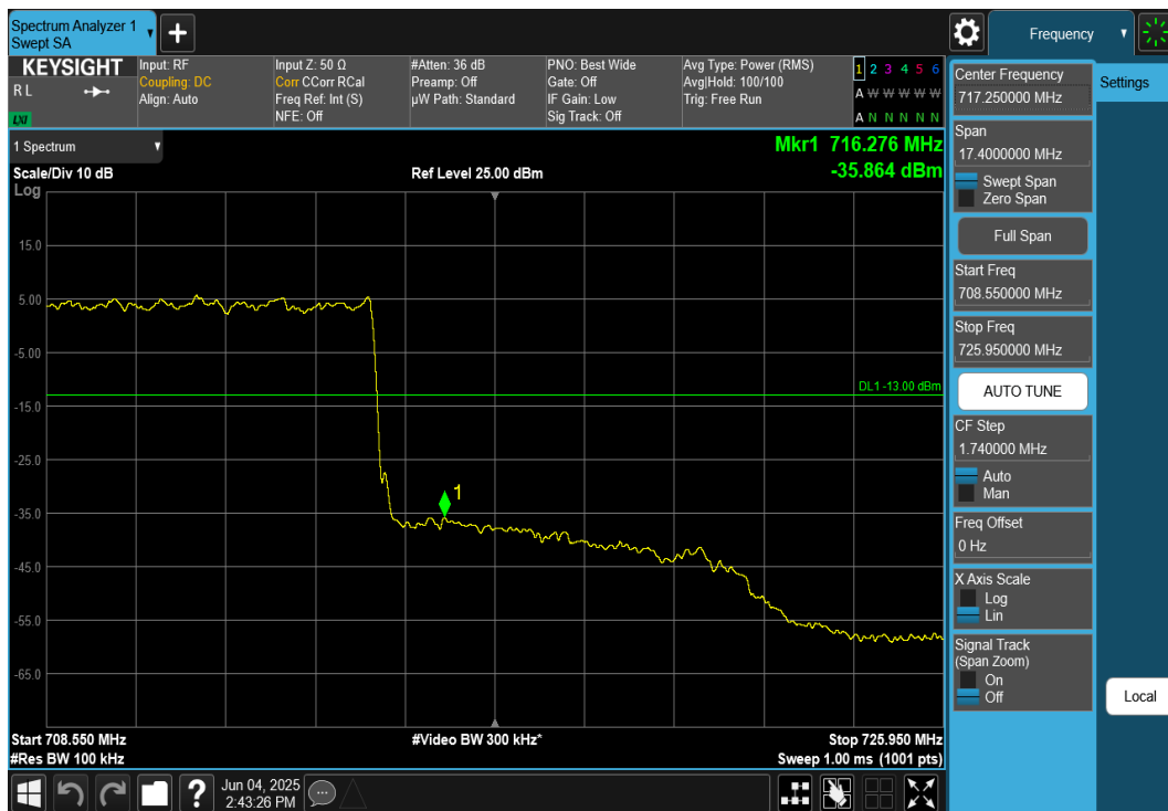
Plot 7-241. Upper Band Edge Plot (NR Band n12 – 15MHz DFT-S-OFDM \pi/2 BPSK - Full RB)
