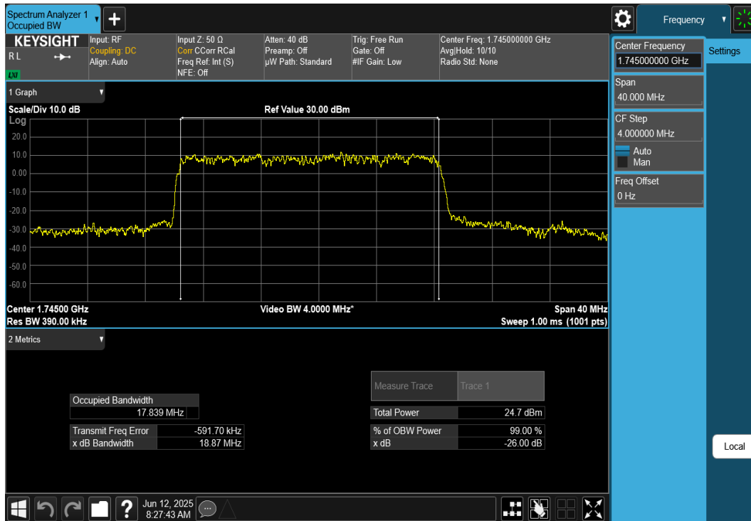
Plot 7-45. Occupied Bandwidth Plot (NR Band n66 - 20MHz DFT-s-OFDM \pi/2 BPSK - Full RB)
