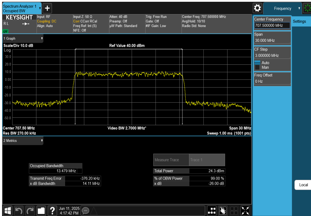
Plot 7-73. Occupied Bandwidth Plot (NR Band n12 - 15MHz DFT-s-OFDM \pi/2 BPSK - Full RB)
