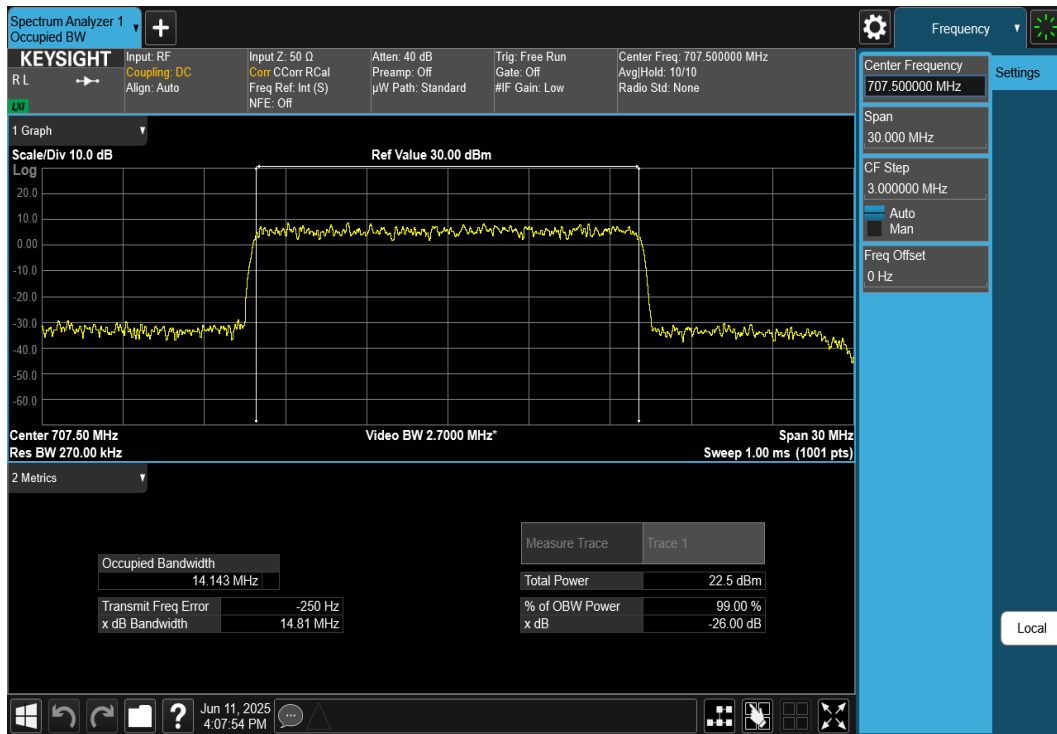
Plot 7-74. Occupied Bandwidth Plot (NR Band n12 - 15MHz CP-OFDM QPSK - Full RB)
