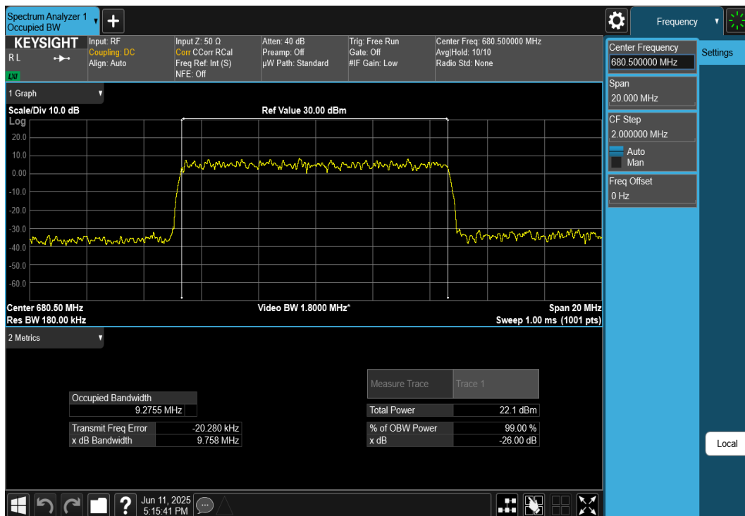
Plot 7-56. Occupied Bandwidth Plot (NR Band n71 - 10MHz CP-OFDM 64-QAM - Full RB)
