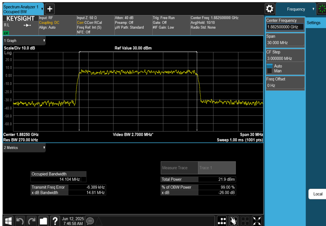
Plot 7-22. Occupied Bandwidth Plot (NR Band n25/n2 - 15MHz CP-OFDM QPSK - Full RB)
